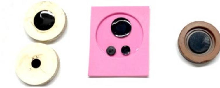
**Figure 6. 2.** Moulds, silicon sheets, and centralizer forms were employed in the manufacturing and installation of the specimen into the DSR
