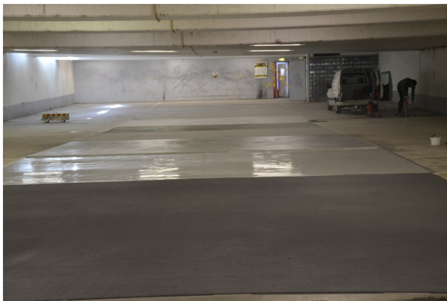
Figure 2.2 Completed total test area with seven coating systems - Åkeshov 2014 (Photo: Y Edwards)
