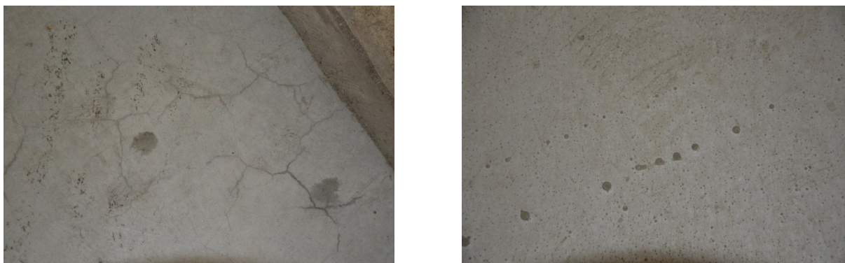
Figure 2.5 Crazing (left hand side) on test area 5 (2016) and pinholes (right hand side) on test area 6 (2015) (Photo: Y Edwards)
