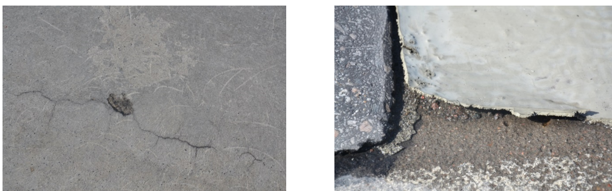
Figure 2.6 Crazing/minor damage (left hand side) on test area 5 (2016) and adhesion loss (right hand side) on test area 4 (2016) (Photo: Y Edwards)
