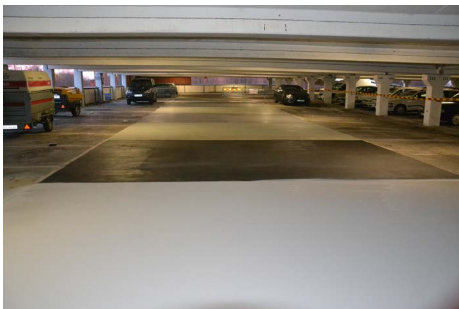
Figure 2.1 Completed total test area with nine coating systems - Kville 2013 (Photo: Y Edwards)
