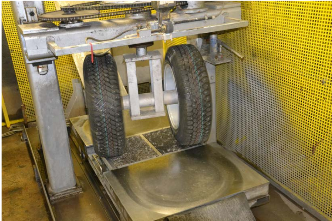
Figure 2.7 Equipment for testing Scuffing resistance, with studded tyres (Photo: Y Edwards)
