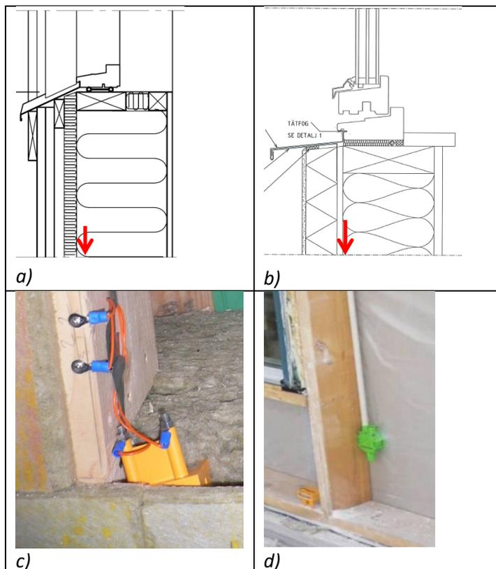
*Figure 2. Vertical cross-section of external walls (a–b) with part of window-wall interface. The outdoor area is to the left. The red arrows show the studied positions. Photo (c) shows the position of a sensor in a residential building of seven-storey height. Photo (d) shows the position of a sensor in a residential building of two-storey height.*
