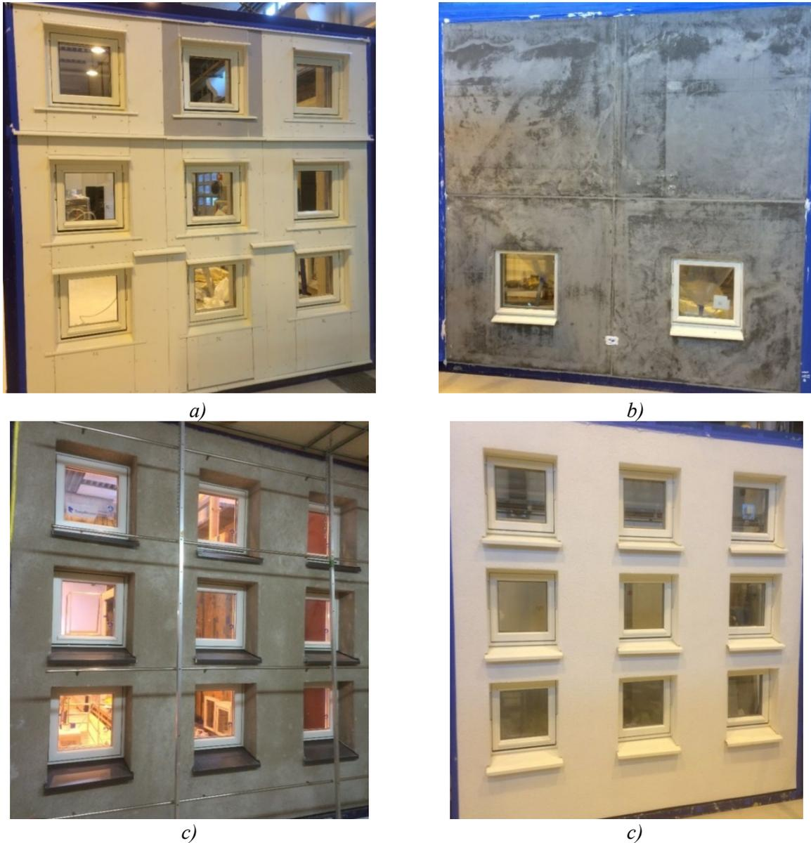
*Figure 4. (a) Ventilated façade with polymer composite boards, (b) 15 mm thin prefabricated high-performance concrete sandwich element with elastic joints, (c) 20 mm plaster façade with 200 mm mineral wool with drainage possibility and weather barrier (second line of defence), (d) 8 mm plaster on 100 mm EPS with drainage possibility and weather barrier. Water spray racks are shown in (c).*
