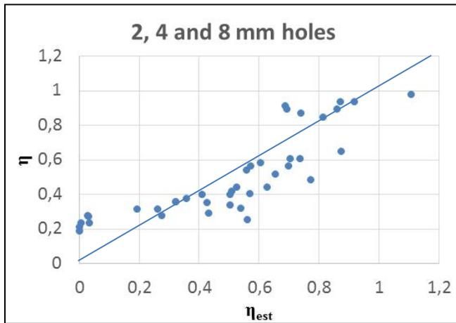
Figure 15. Factor  $\eta$  (measured) is shown on the vertical axis and  $\eta_{est}$  (estimated) on the horizontal axis for 2, 4 and 8 mm holes in fiber cement board without dams, and comparison to the optimal line. The line corresponds to when estimated values exactly correspond to measured values. The water flow on the façade of 2.9 l/min,m.
