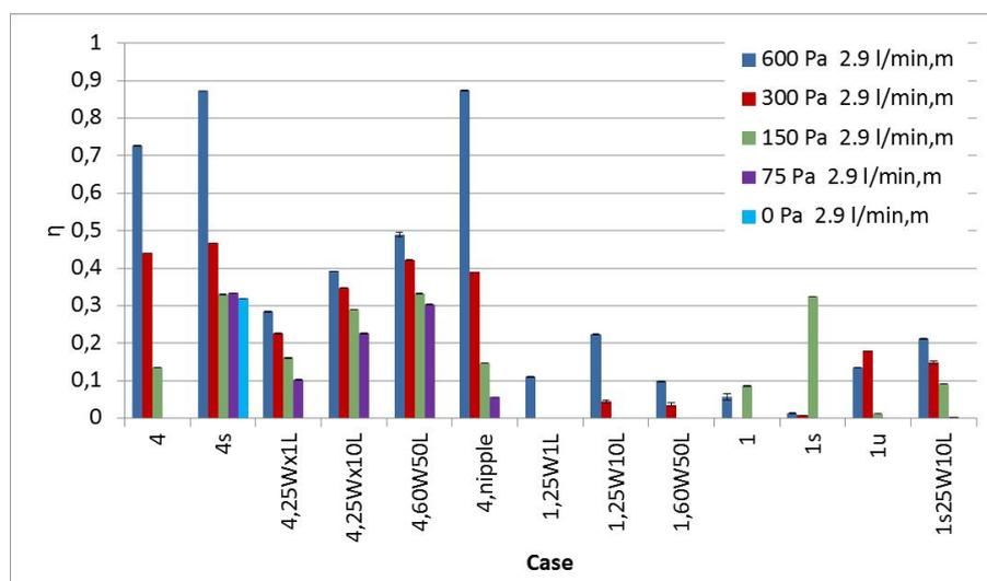
Figure 14. The  $\eta$ -factor of the measured values. Holes with and without dam in polycarbonate board. Water flow on the façade of 2.9 l/min,m.
