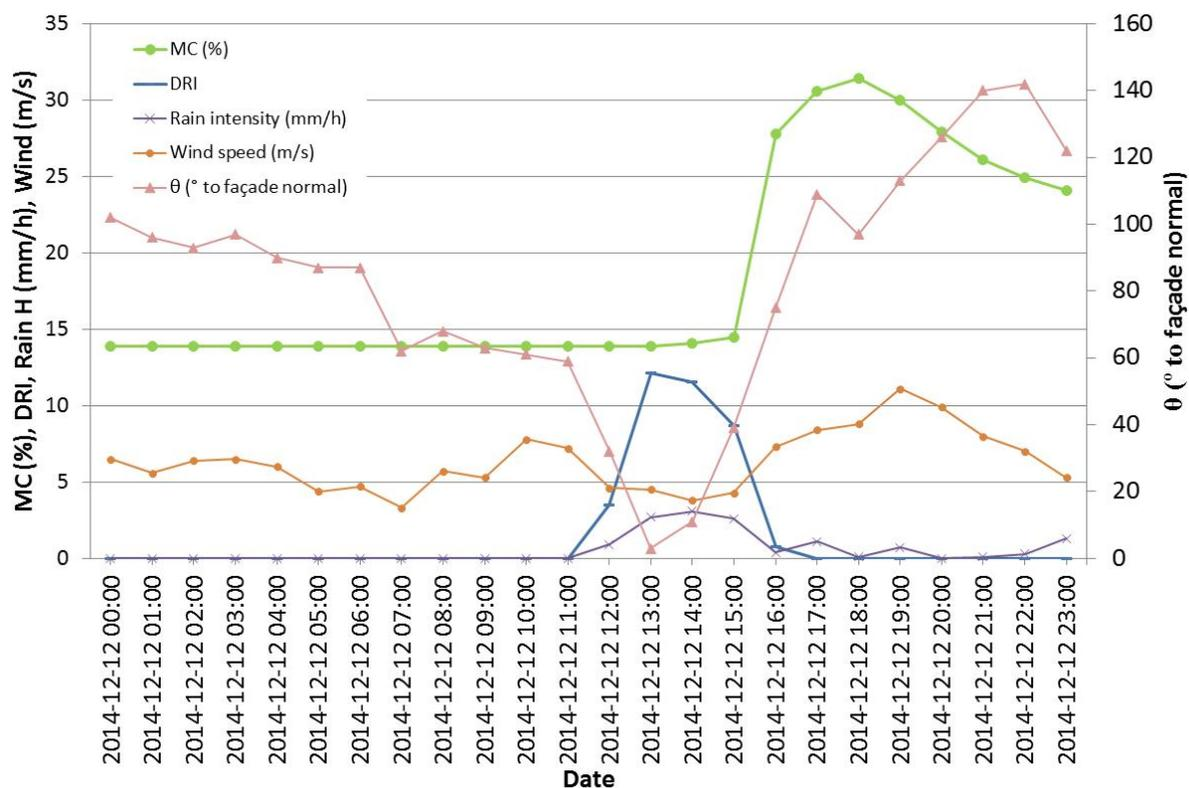
Figure 9. Diagram of one of the days in Figure 8. Driving rain index, DRI (-), rain intensity on horizontal surface (mm/h), wind speed (m/s) and wind direction ( $\theta$ ) are from a nearby weather station. If wind direction is towards the façade, normal vector of the façade, the angel is zero in the diagram.
