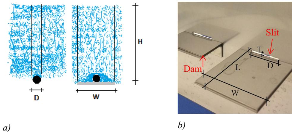
Figure 1. (a) Catch area as regards hole width ( $D$ ) or dam width ( $W$ ) plus façade height ( $H$ ). The assumed catch area is shown within the two vertical lines. (b) The figure shows a vertical stainless steel sheet with several horizontal stainless steel dams located underneath of defects consisting of horizontal slits. Further descriptions of dimensions are given with notations such as protrusion length ( $L$ ) and height ( $T$ ) of slits, as used in Chapter 5.
