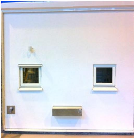
*Figure 3. Example of a commercial test wall (size 3 x 3 m) with façade details; windows, balcony, and two fixings (marquis and downpipe fastener).*
