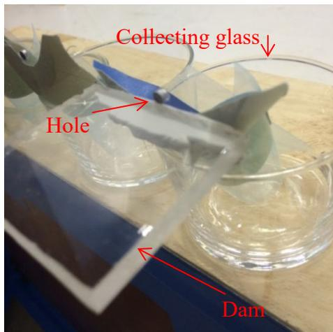
*Figure 7. A horizontal dam mounted beneath a hole in a polycarbonate board (note that the polycarbonate board is transparent and located in front of the glasses). Parts of the other cases are also visible further away in the photo as well as collecting channels behind the polycarbonate board. The holes and dams are placed at the bottom of the rain exposed surface. The height of the rain exposed surface was 1 metre.*
