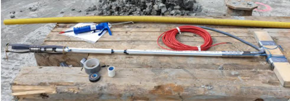
Figure 4.24: *Assembly of vibrating wire extensometer including spider anchor legs before installation 2019-07-02.*
