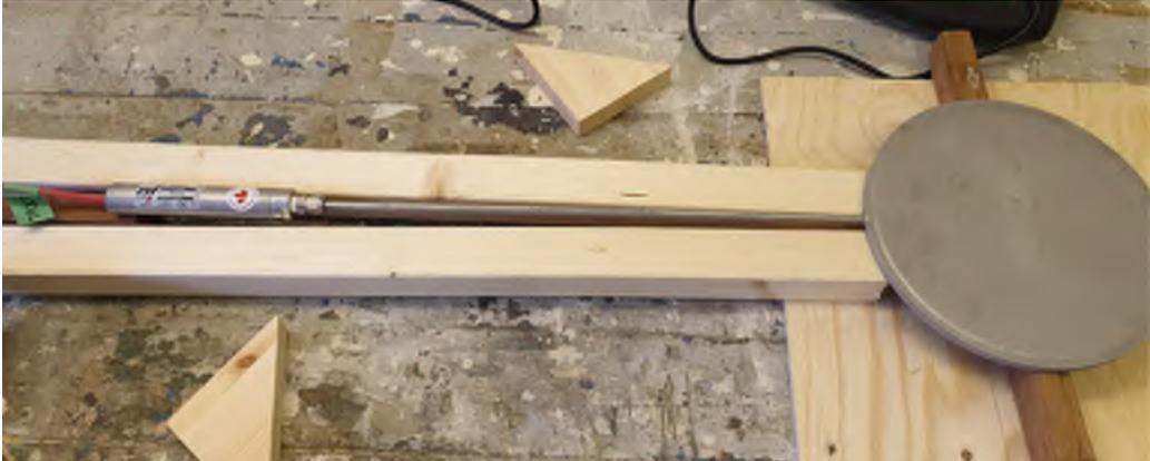
Figure 4.25: *Photo of total earth pressure cell.*
