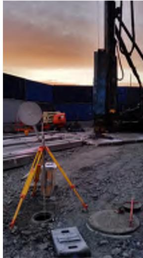
Figure 4.23: Customized tripod for measurements of vertical displacements in bellow-hose "floating" in the clay layer. The reference level of the tripod was established by surveying for each measurement setup, 24 in total.
