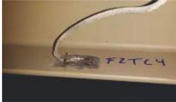
Figure 9. TC welded to the lower chord of truss F2.
