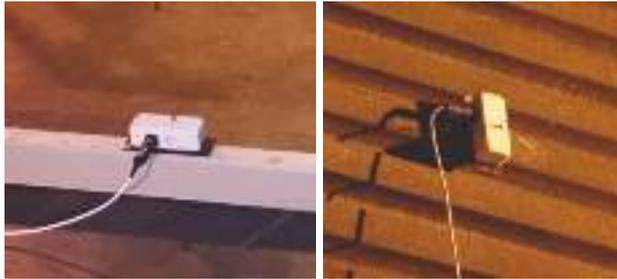
*Figure 13. Displacement meters attached to the beam parallel to and directly under F2 for vertical measures (left) and to the wall of the burn hall for horizontal measures (right).*
