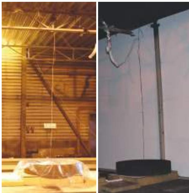
*Figure 8. Figure to the left shows the TC tree mounted centrally over the fuel pan just before test 1. In the same figure, parts of Truss F2 and F1 in the experimental setup can also be seen as well as the wall and column in the background which are not part of the test construction but a part of the burn hall itself. The figure to the right shows the TC tree mounted centrally over the fuel pan before test 3.*
