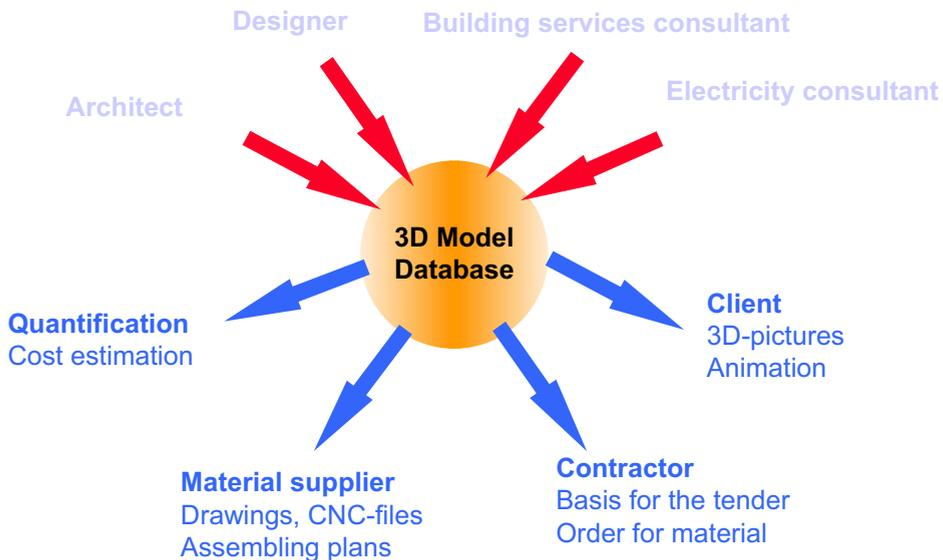
**Figure 6-1: The 3D database model for construction**
