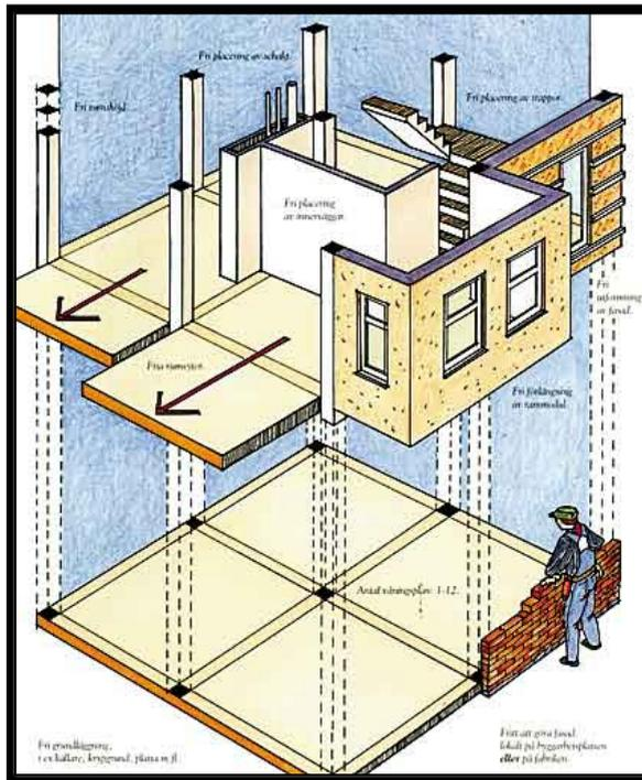
**Figure 5-5: Structural system of the Open House system**
