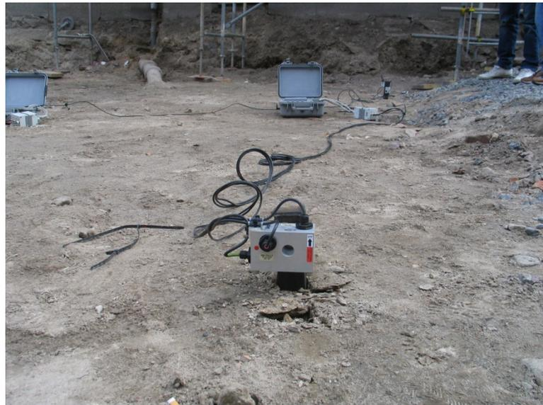
Figure 4. A tri-axial geophone in front and the recorder in the background.
