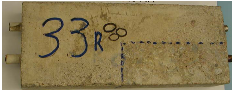
Figure 2. One repaired and reinforced concrete specimen in this investigation. The rectangle to the right is the repair concrete and the rest is the substrate concrete.
