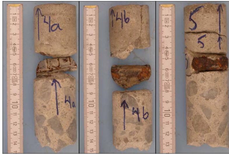
Figure 18. Concrete samples from patch repairs in parking structure Plankan with corroded reinforcement in the transition zone.
