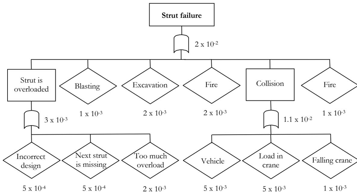
Figure 4.5 Fault tree for the damage event "Strut failure" (after Olsson 1998).
