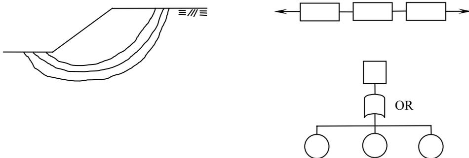
Figure 2.8 System selection considerations of a slip surface – reliability block diagram and fault tree (modified after Carlsson et al. 2004).
