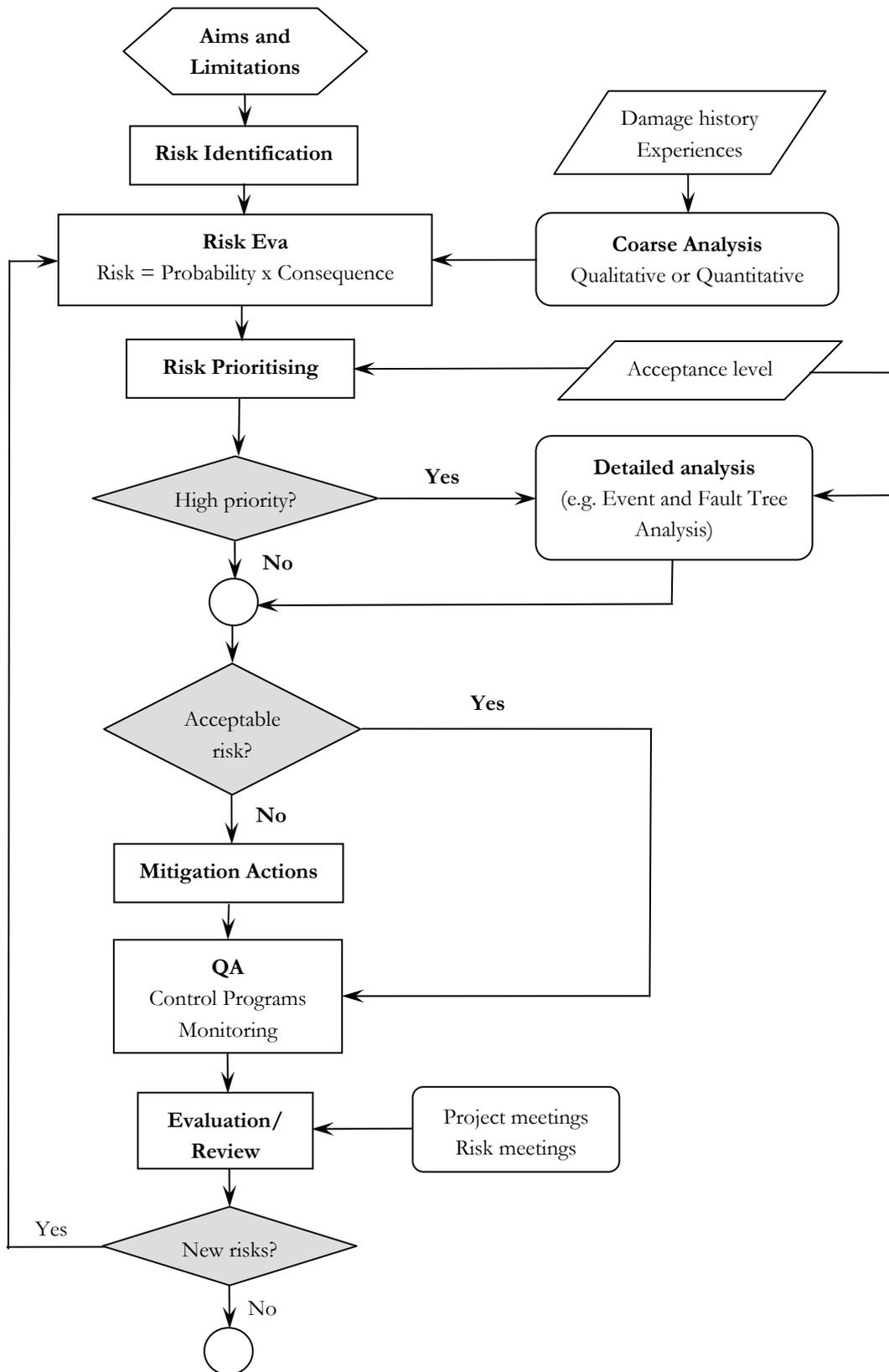
Figure 4.3 The risk management process in the South Link Road Construction (Swedish Road Administration 2002).
