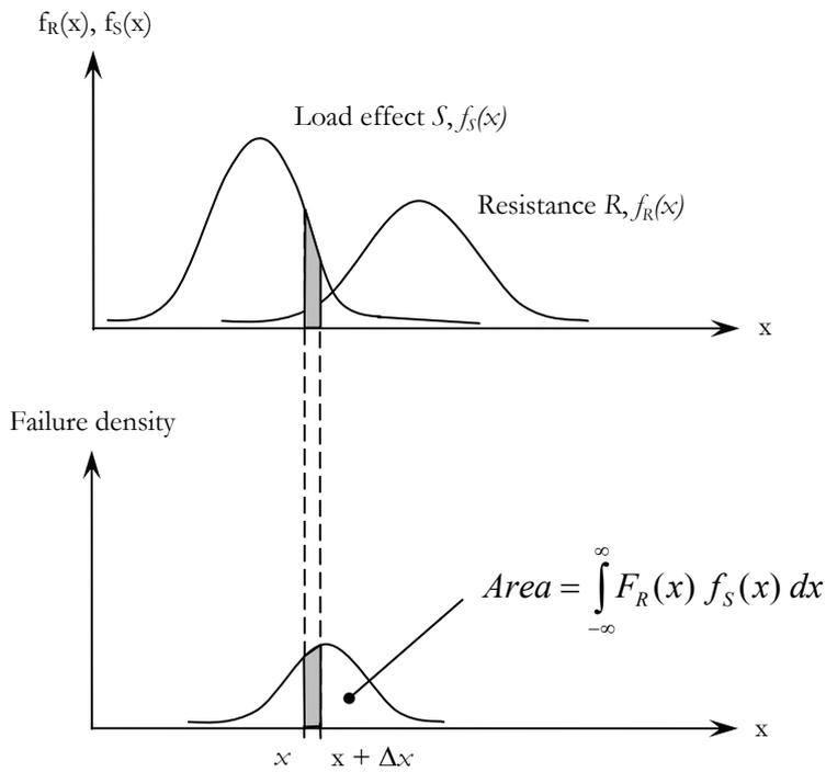
Figure 2.6 Basic R–S problem, a  $f_R(x)$  and  $f_S(x)$  representation (Melchers 2002).
