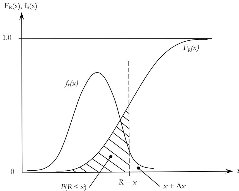
Figure 2.5 Basic R-S problem, a  $F_R(x)$  and  $f_S(x)$  representation (Melchers 2002).
