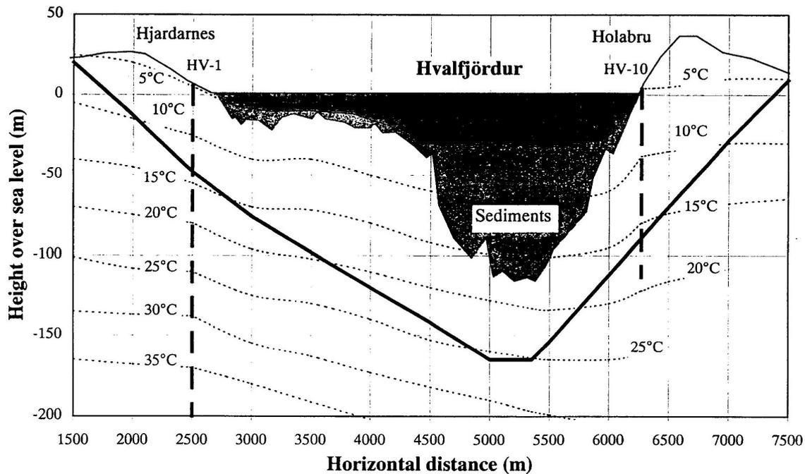
Figure 4.12 Longitudinal cross section of the tunnel with expected temperature conditions (Tengborg et al. 1998).
