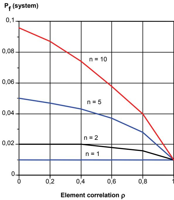
Figure 2.7 Probability of failure for a series system with  $p_i = 0.01$  as a function of the correlation coefficient  $\rho$  and the number of elements  $n$  (Thoft-Christensen & Baker 1982).
