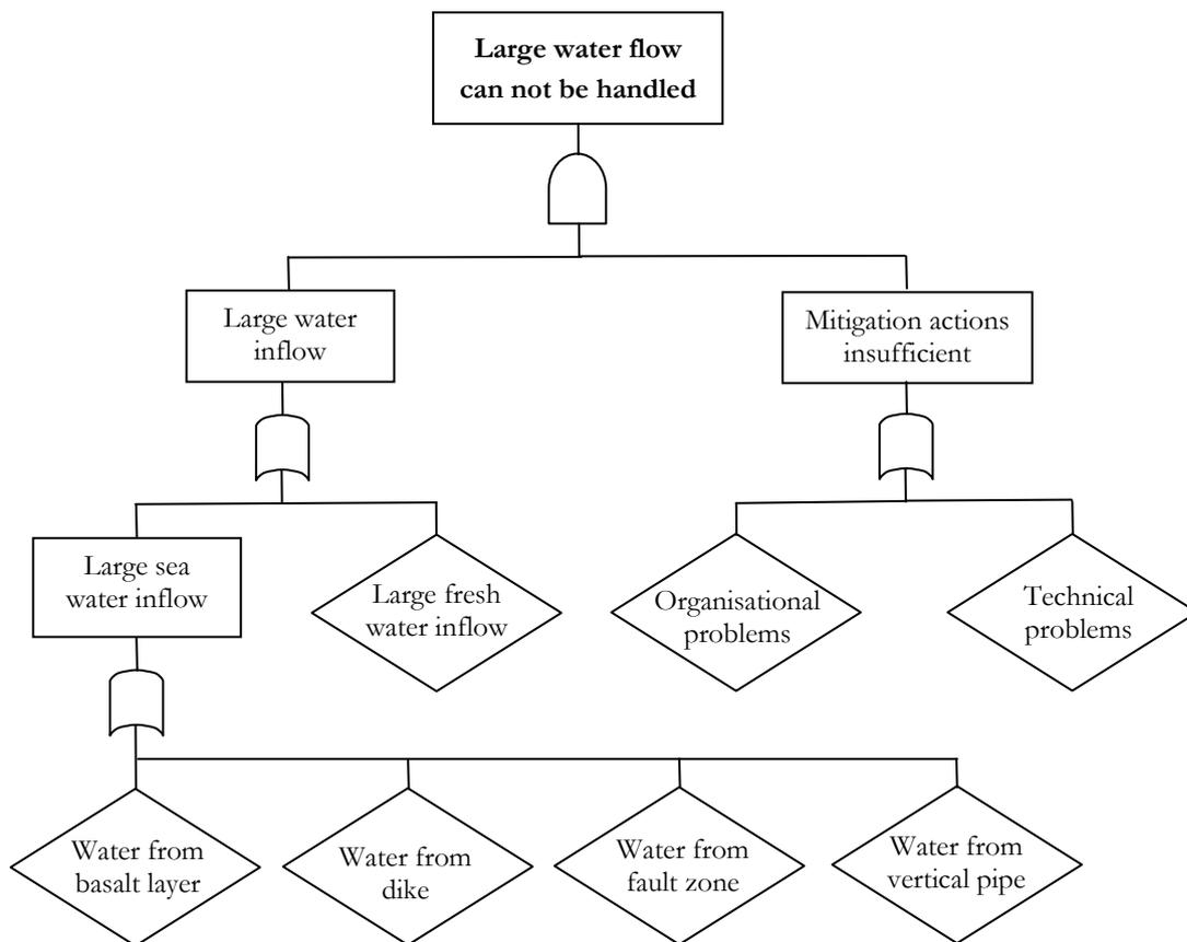
Figure 4.14 Fault tree for the most crucial damage event (after Olsson et al. 1996).
