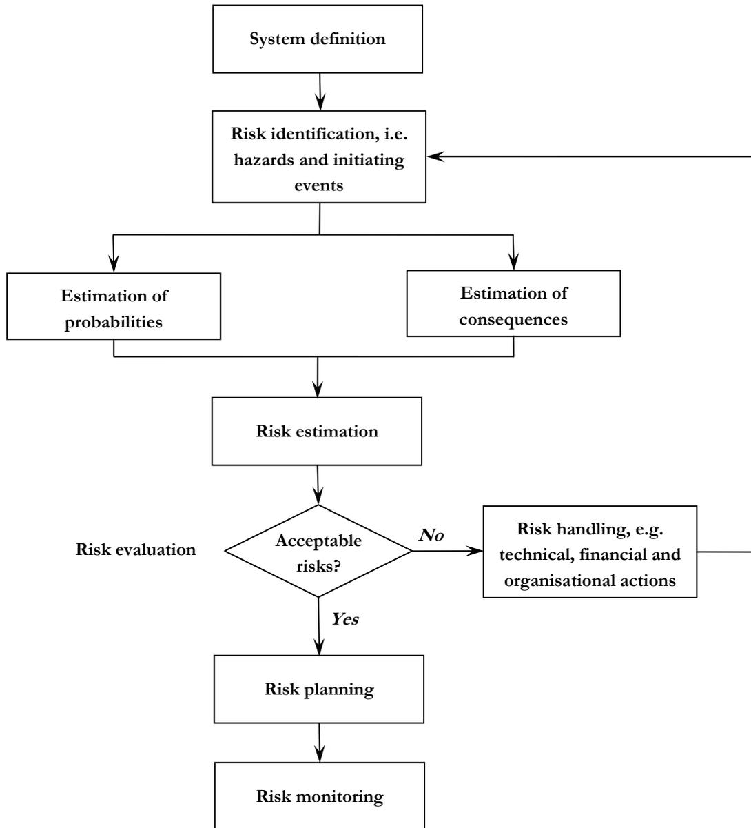
Figure 2.3 The structure of the risk management process (after Hintze 1994 and IEC 1995).
