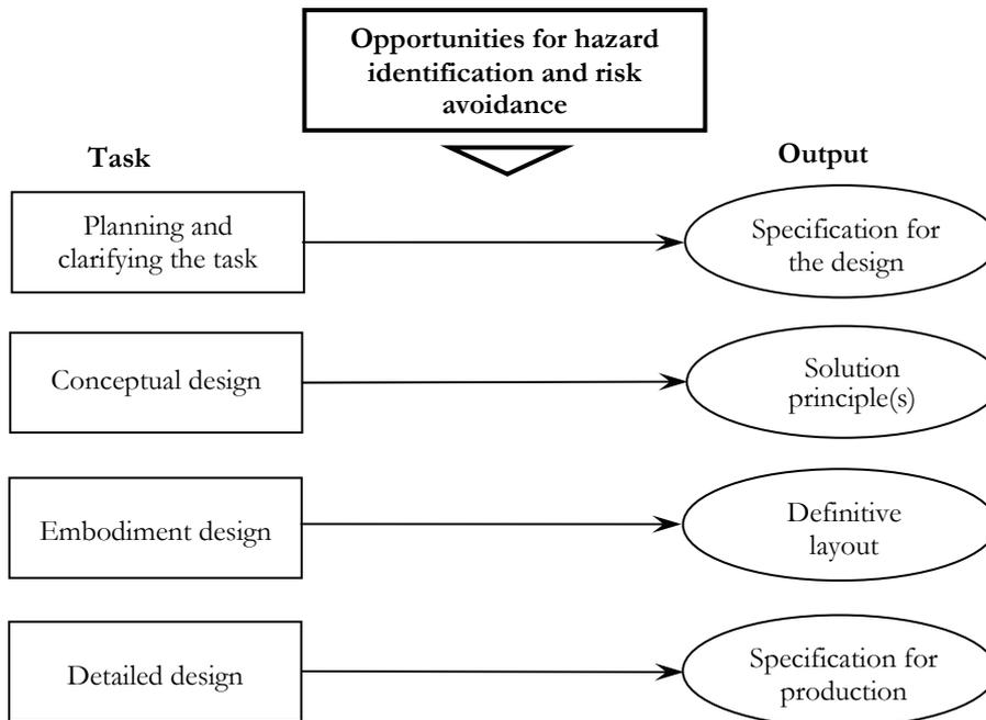
Figure 5.1 Elements of systematic engineering design (Pahl et al. 1996).
