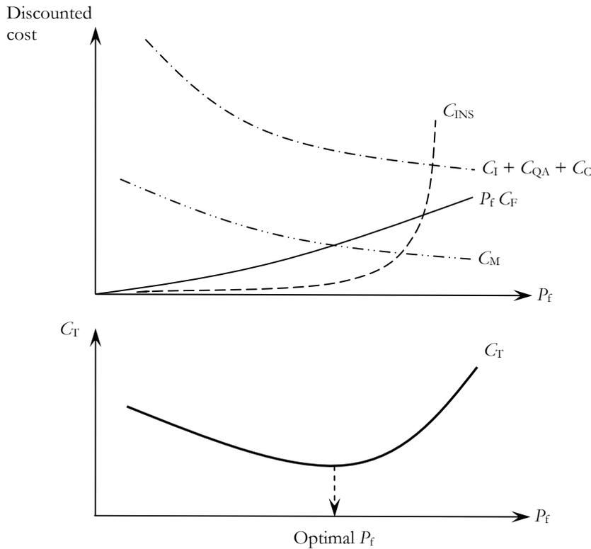
Figure 2.28 (a) Component cost and (b) total cost as a function of  $p_f$  (after Melchers 2002).
