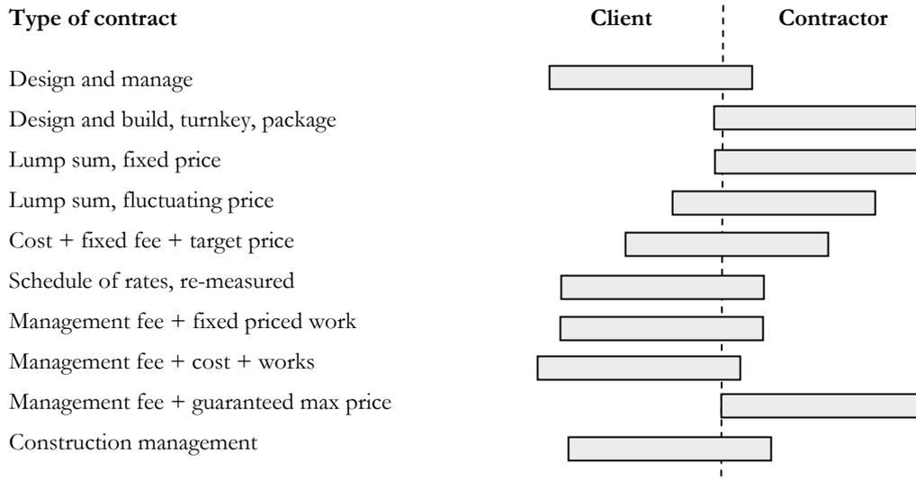
Figure 3.4 Risk sharing between the client and the contractor depending on the type of contract (Flanagan & Norman 1993).
