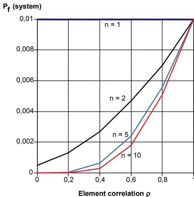
Figure 2.9 Probability of failure for a parallel system with ductile elements with  $p_i = 0.01$  as a function of the correlation coefficient  $\rho$  and the number of elements  $n$  (Thoft-Christensen & Baker 1982).
