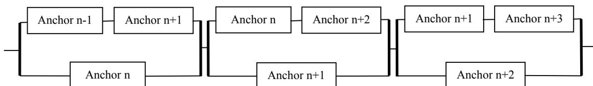
Figure 2.13 Reliability block diagram of an anchor system (Carlsson et al. 2004).
