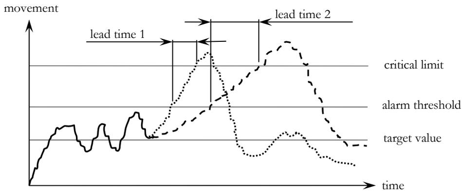
Figure 3.10 Alarm thresholds and lead times for two different stress-strain relationships A and B (after Paté-Cornell & Benito-Claudio 1987).
