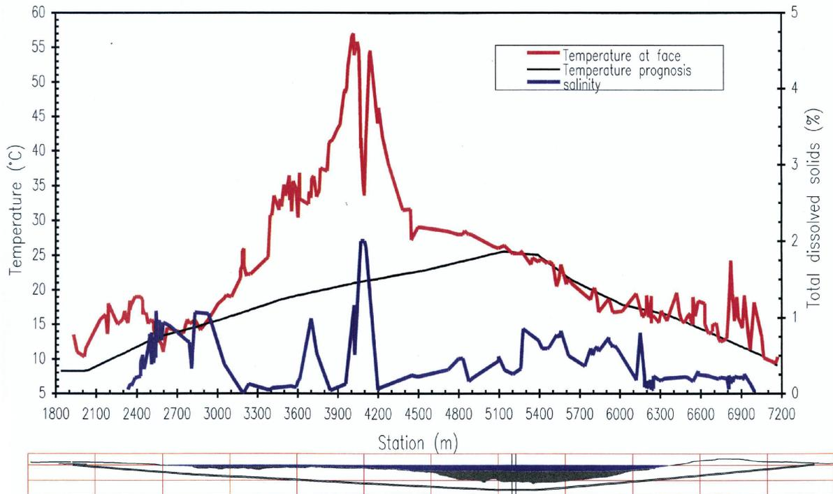
Figure 4.16 Result of the measurement of water temperature in the tunnel (Tante 1998).
