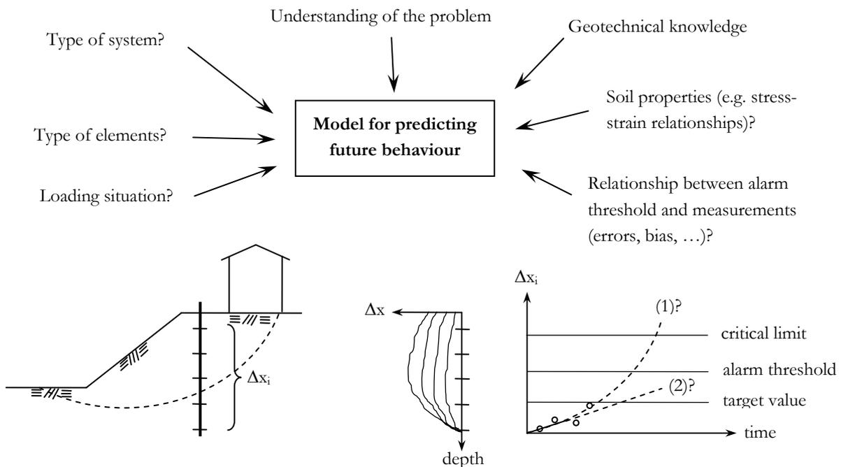
Figure 3.11 Model for predicting future behaviour in order to decide corrective actions and alarm values (modified after Olsson & Stille 2002).
