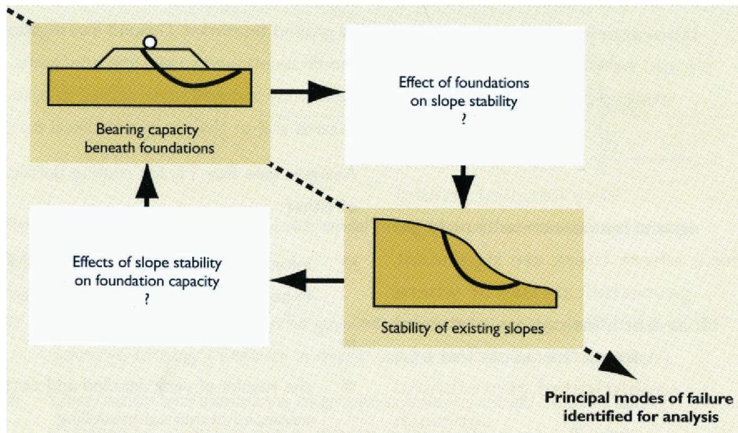
Figure 5.2 A system approach, using interaction matrices, to identify unfavourable design interactions (Clayton 2001b).
