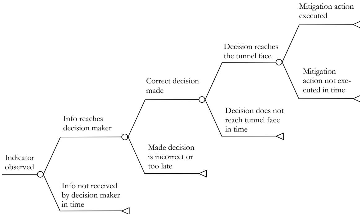
Figure 4.15 Event tree for the chain of events from indication of a hazard to the execution of a pre-determined mitigation action (after Olsson et al. 1996)
