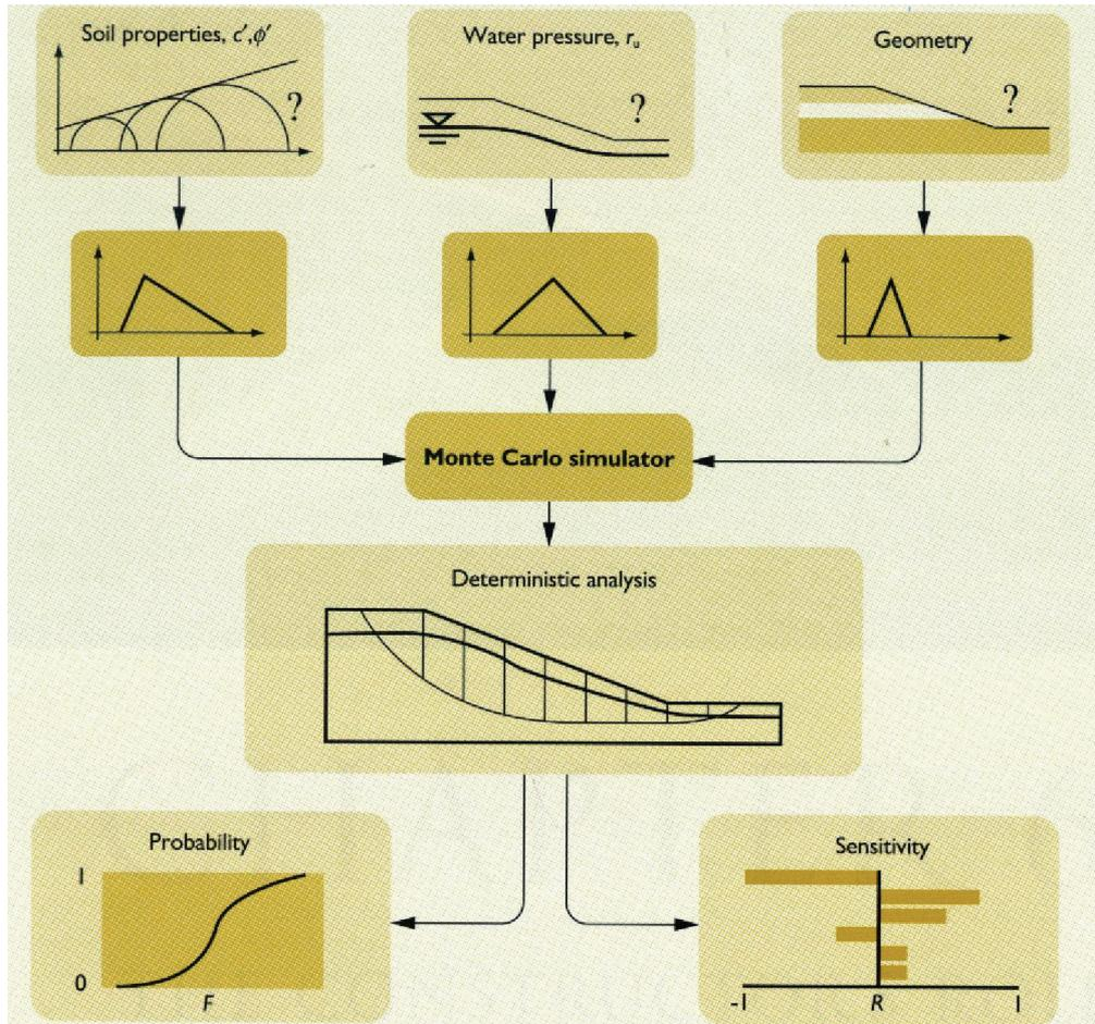
Figure 5.3 An example of sensitivity analysis of a slope (Clayton 2001b).
