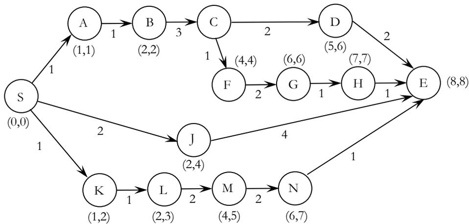
Figure 3.7 Critical path resulting from the roll-forward-roll-back algorithm (Bedford & Cook 2003).
