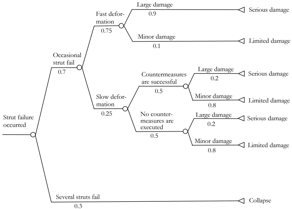
Figure 4.6 Event tree for damage on residential block “Asplången” assuming that strut failure has occurred (after Olsson 1998).
