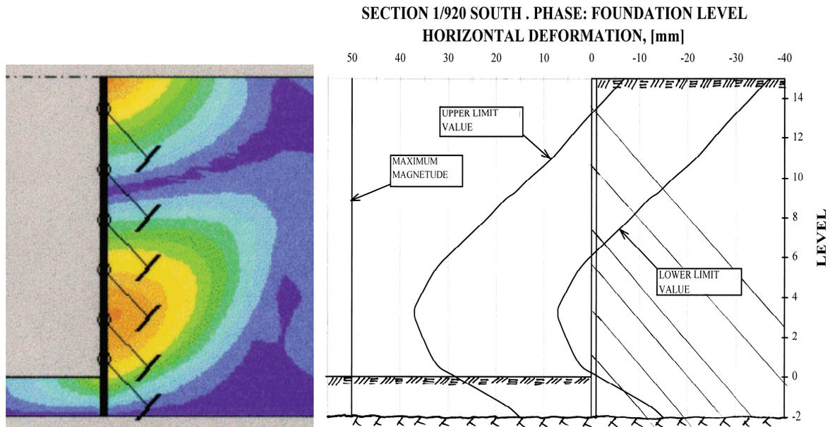
Figure 4.7 Alarm thresholds and critical limits for the horizontal deformation of the sheet pile wall in section 1/920 south (Hintze 2001).
