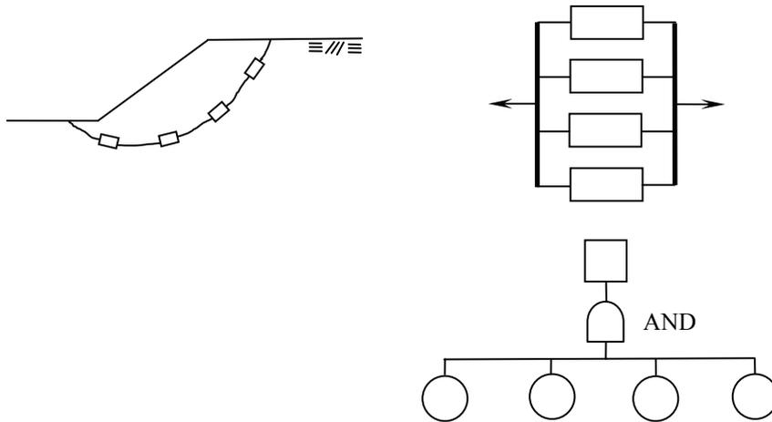
Figure 2.10 System selection considerations of a slip surface – reliability block diagram and fault tree (modified after Carlsson et al. 2004).
