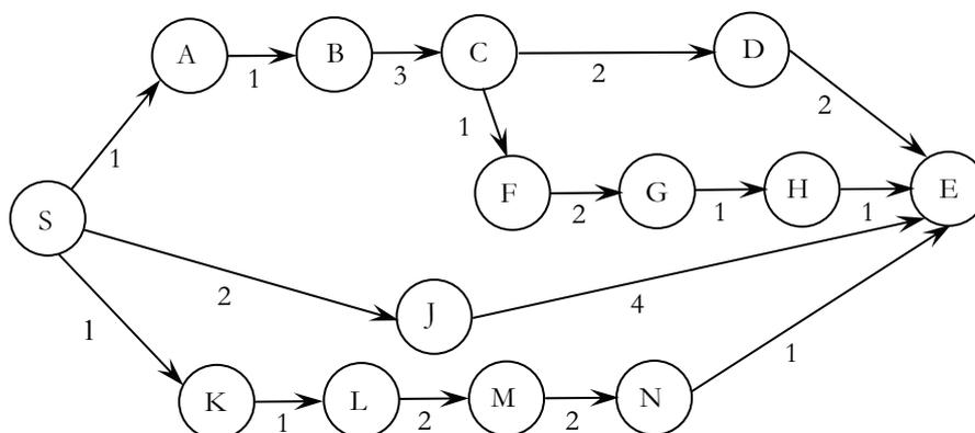
Figure 3.6 A simple network diagram with required times for completing the work activities (Bedford & Cook 2003).
