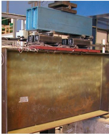
Figure 3.4 Photo of the P1440 test with the load distributing beams on top of the girder.
