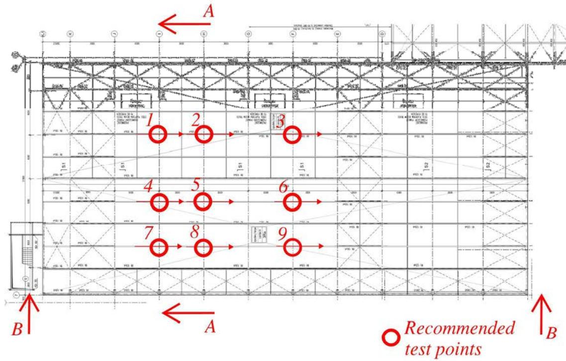
Figure 4.3: Examples of recommended testing points in a slender roof structure, plane view.
