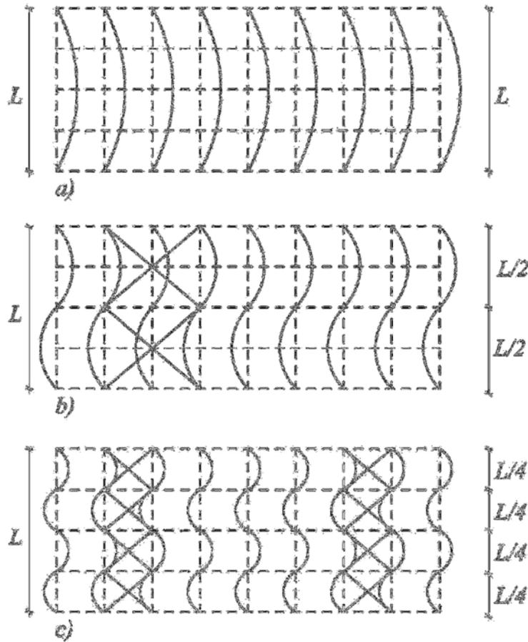
Figure 3.15: Different buckling modes of primary roof members dependent upon the bracing configuration that is found, where a) involves there being no bracing in the plane of the roof, the buckling length being equal to  $L$ , b) the wind trusses reducing the buckling length to  $L/2$ , and c) the wind trusses reducing the buckling length to  $L/4$ .
