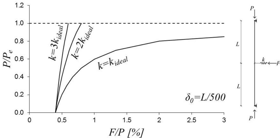
Figure 3.13: The relationship between the force that is applied and the corresponding bracing force of a braced strut obtained for three different values of the bracing stiffness,  $P$  is the load that is applied,  $P_e$  is the Euler load ( $\pi^2 EI/L^2$ ),  $k_{ideal}$  is the ideal stiffness of the bracing ( $2P_e/L$ ),  $L$  is the distance between successive restraints, and  $F$  is the bracing force.
