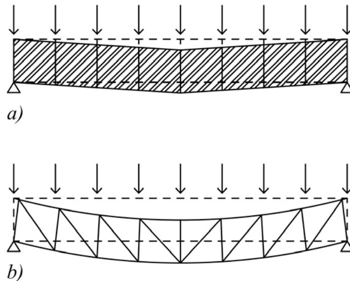
Figure 3.17: Deformations of the roof section of the stabilizing bay of a roof structure, a) when using a decking, so that diaphragm action takes place, the displacement is basically due to pure shear (the bending deformations that occur are usually neglectable), and b) when a wind truss is employed, the displacement then is a combination of shear and of bending displacements.
