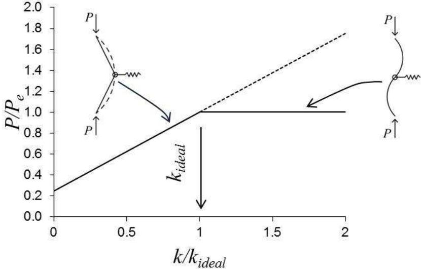
Figure 3.9: The elastic buckling capacity of a braced strut shown as a function of the brace stiffness,  $k_{ideal}$  is the ideal bracing stiffness, and  $P_e$  is the the Euler buckling load when buckling between successive restraints occurs.
