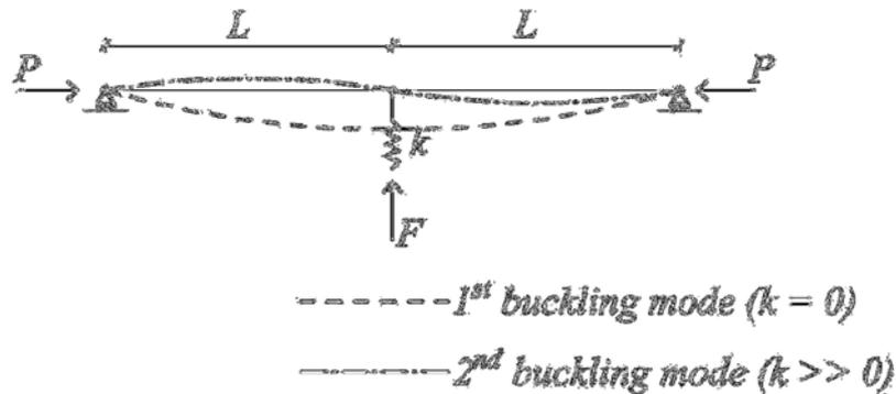
Figure 3.7: A braced strut.
