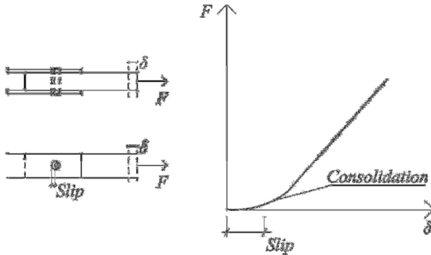
Figure 3.19: Potential slip in bolted connections due to the holes being oversized.
