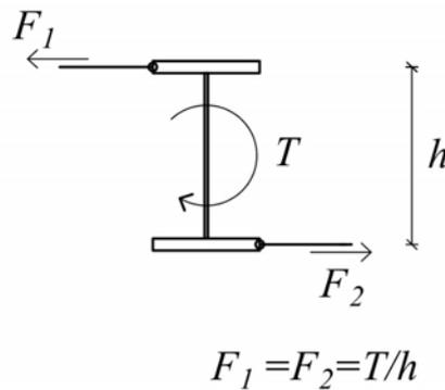
Figure 3.6: Torsional bracing of an I-girder as achieved by means of two translational bracings, i.e. by the force couples  $F_1$  and  $F_2$ . It is assumed that the bracings can take both tension and compression.
