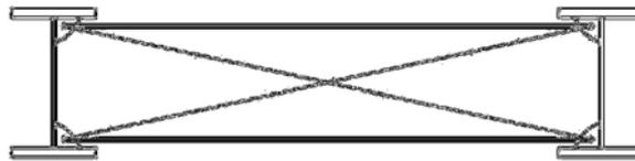
Figure 3.4: The relative bracing of two steel girders, both torsionally and translationally.
