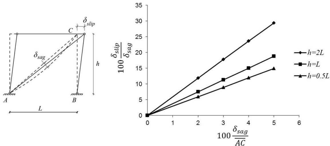
Figure 3.22: An example of how the sag of a diagonal member would require that a movement ( $\delta_{slip}$ ) at the top of the frame take place in order for the diagonal to be activated (i.e. straightened out).
