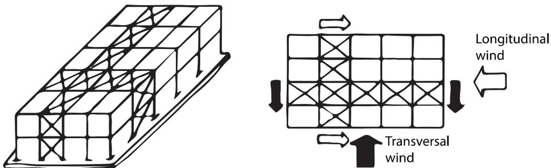
Figure 3.14: Lateral stabilization of a hall type building (Klasson, 2015).
