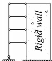
Figure 3.2: Discrete bracing of a column.
