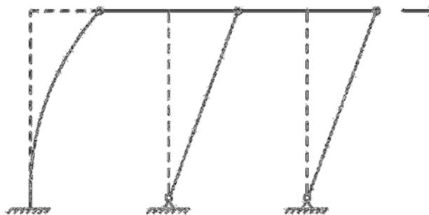
Figure 3.5: A lean-on system of columns.
