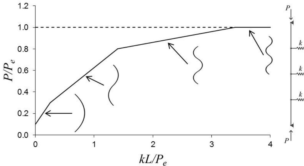
Figure 3.10: Plot of the buckling load  $P$  in relation to the bracing stiffness of a braced strut, where  $k$  is the bracing stiffness,  $L$  is the distance between successive restraints and  $P_e$  is the the Euler buckling load when buckling between successive restraints occurs.
