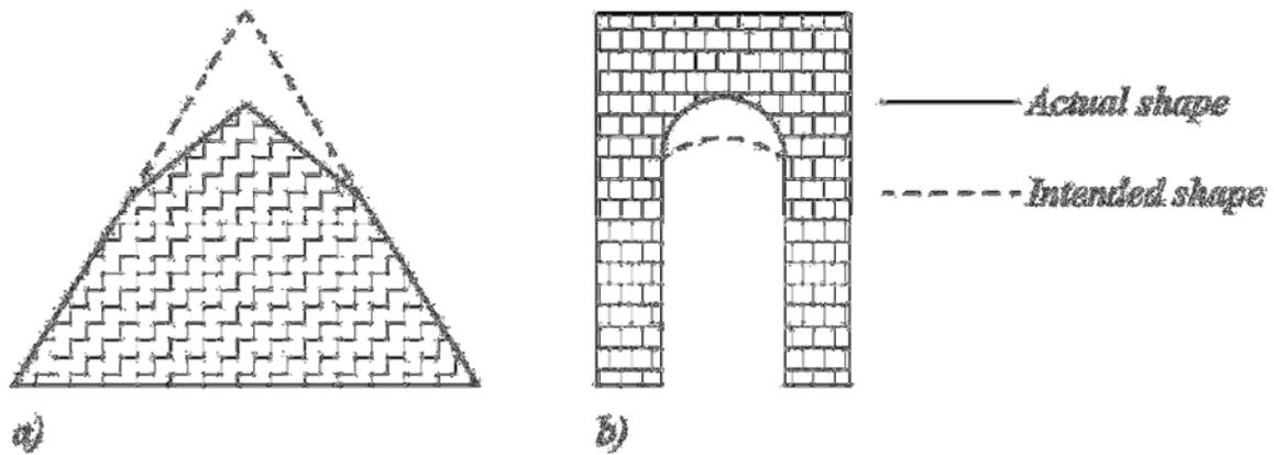
Figure 2.1: Examples of how principles of trial and error may have decided the design of ancient buildings: a) the angle of a pyramid, and b) the radius of an archway.
