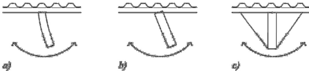
Figure 2.9: A primary beam in a roof structure rotating around its longitudinal axis due to negative bending: a) torsional rigidity being provided by the purlins and the roof cladding, b) the joint between the primary beam and the purlin being a pinned one, and c) torsional bracing of the cross section being provided by means of tension ties connected to the bottom side of the member.
