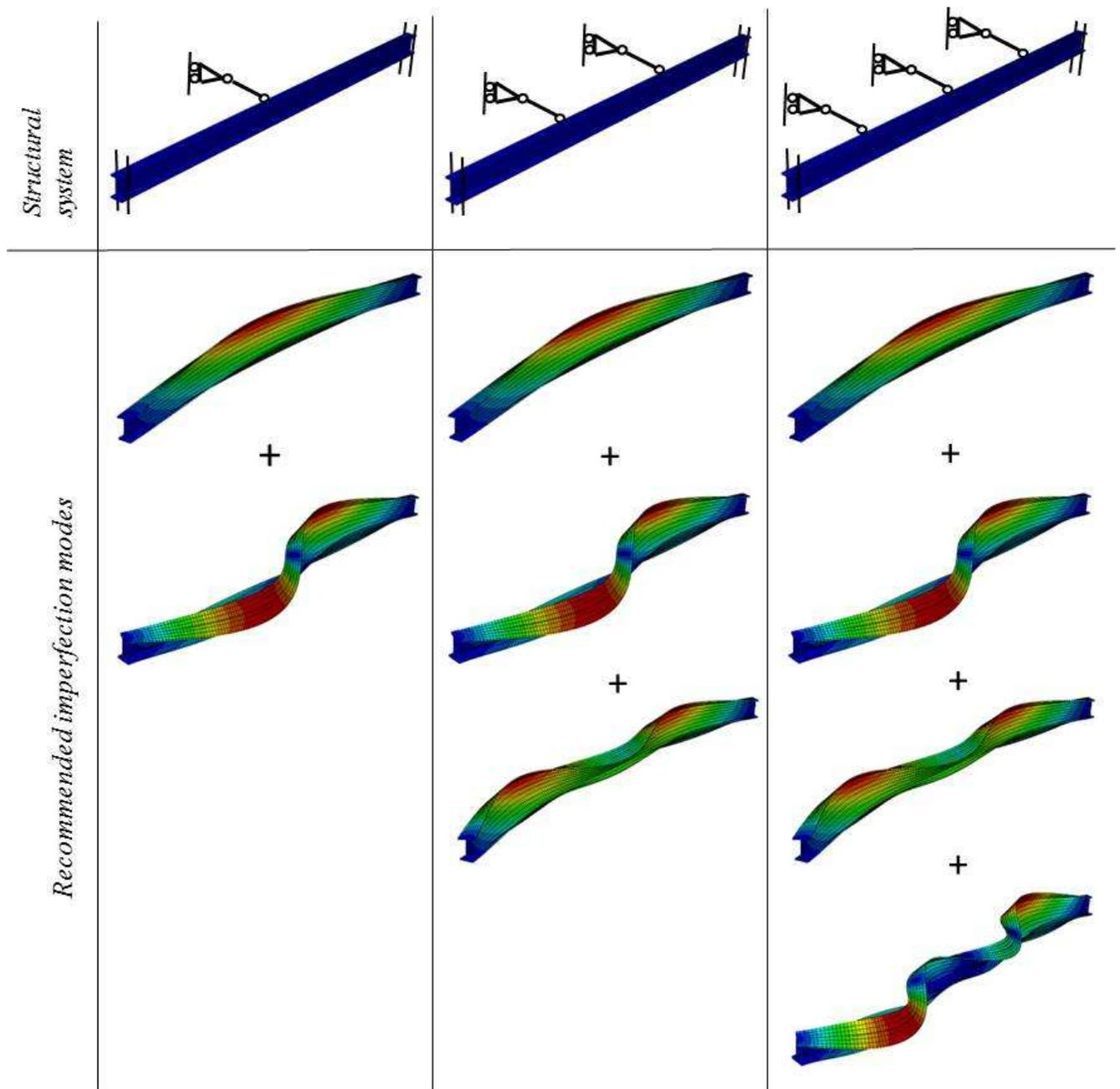
Figure 3.18: Recommended imperfection modes intended for inclusion in the imperfect shape of three different braced beams, 1) with a simply supported beam with one intermediate bracing, 2) with two intermediate bracings, and 3) with three intermediate bracings.
