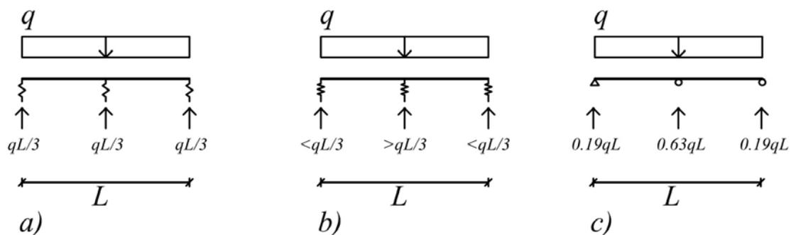
**Figure 2.4:** A uniformly loaded beam held up by three supports: a) supports of very low stiffness in relation to the bending stiffness of the beam, b) moderately stiff supports, and c) rigid supports.
