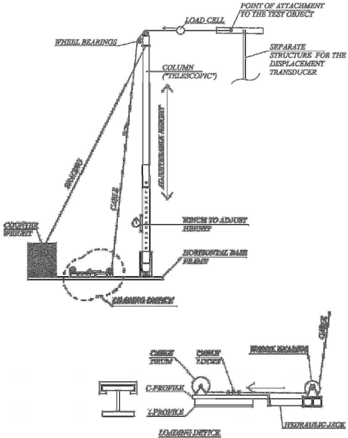
Figure 4.6: A drawing of the test rig.
