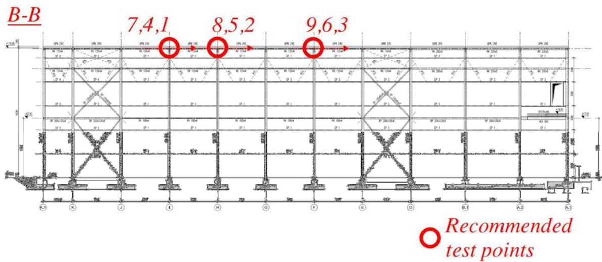
Figure 4.5: Examples of recommended testing points in a slender roof structure, at cross section B-B (see Figure 4.3).
