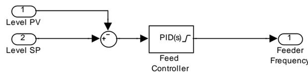
Figure 19. PID controller for the feeder frequency in MATLAB/Simulink.
