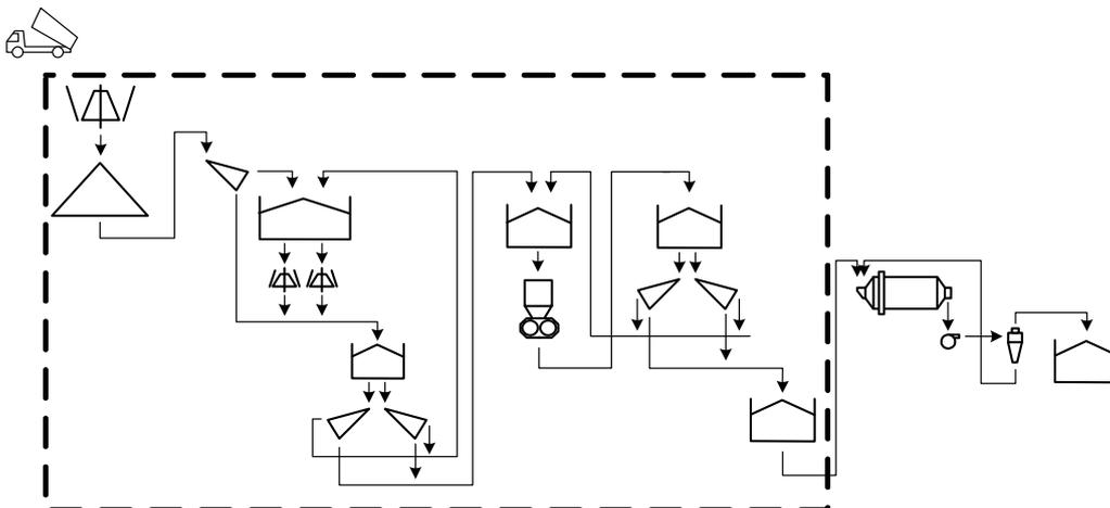
*Figure 6. The focus of this is the crushing and screening stage in aggregate and mineral plants alike, depicted in the dashed box.*
