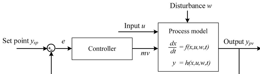
Figure 18. General representation of a feedback control loop. Modified from Marlin [51].
