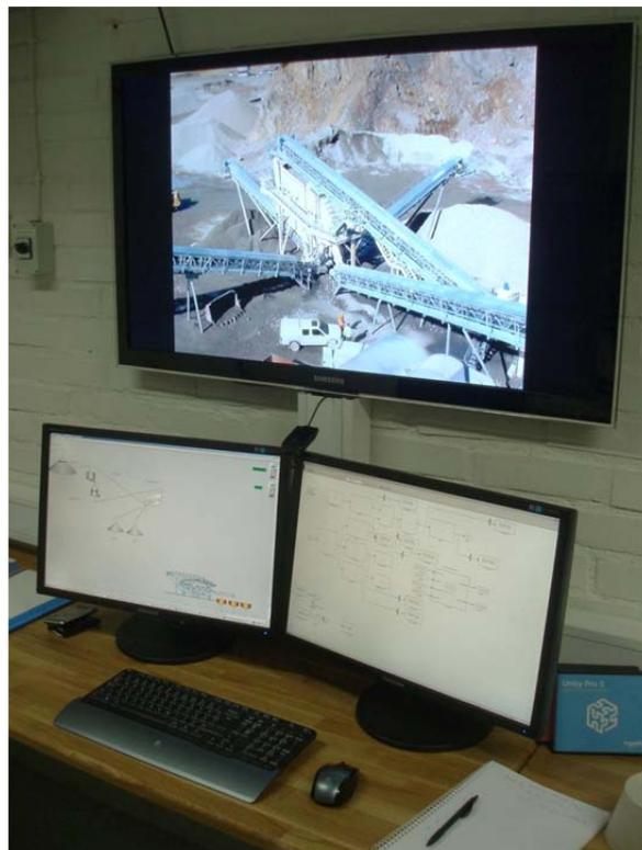
*Figure 39. The simulation computer running a plant simulation while information is being transferred to the operator's screen.*
