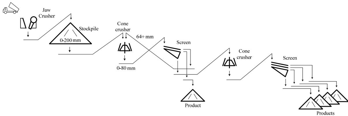
Figure 1. A crushing plant in an aggregate application.
