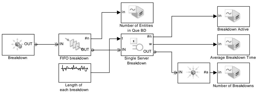
Figure 17. Event generated with SimEvents for representing a mechanical breakdown.
