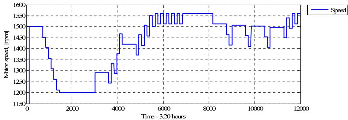
Figure 38. Simulation results after the optimization. The upper graph illustrates the mass-flow on different conveyors while the lower one illustrates the change in speed set point during the simulation.
