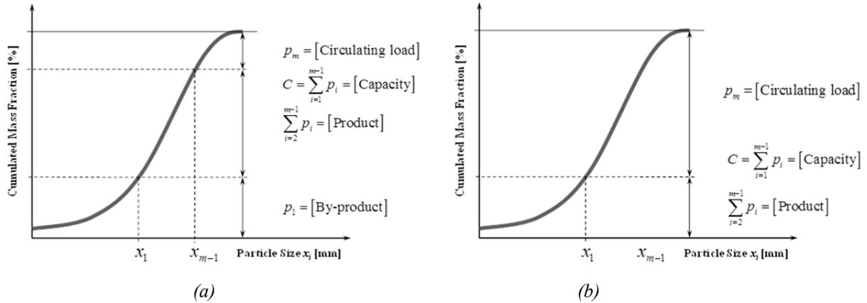
Figure 4. Schematic illustration of capacity, product, circulating load and by-product identified on a particle size distribution for aggregate (a) respectively mining application (b), as presented by Lee [6].
