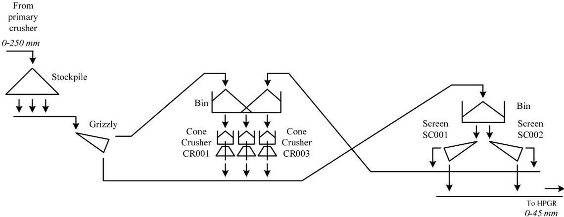
Figure 28. Flowsheet of the crushing section of the platinum processing plant as presented in Paper B.
