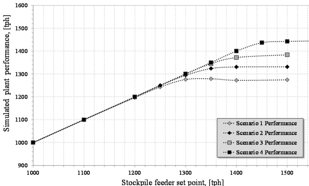
Figure 35. Average plant performance for different feed rates and plant configuration.
