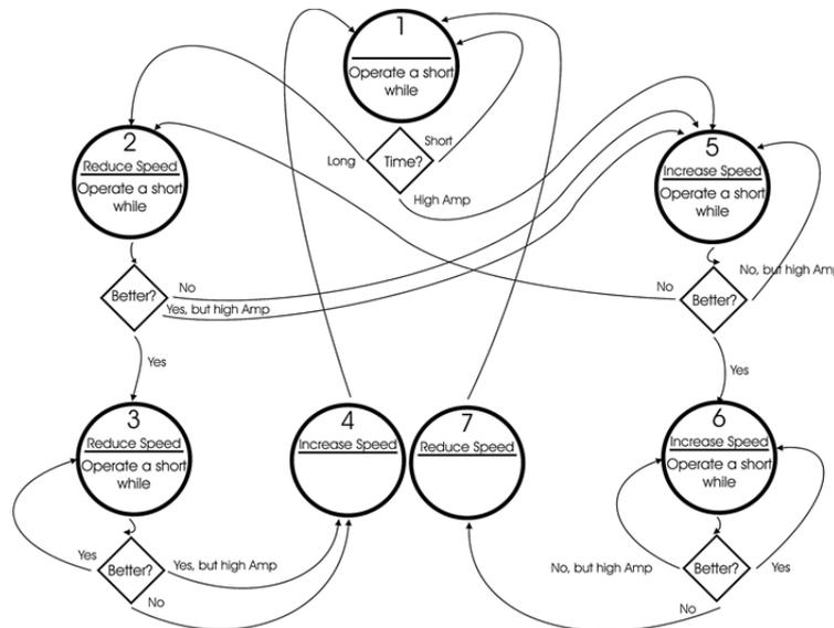
Figure 32. The FSM used for selecting appropriate speed [10].
