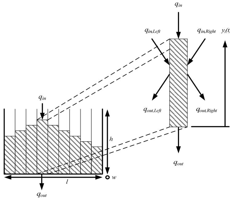
Figure 13. Principle idea with the developed bin model.
