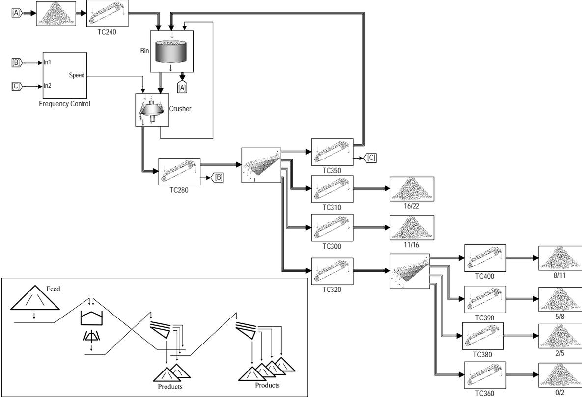
Figure 33. The modelled process in MATLAB/Simulink and the simplified layout of the plant in the embedded picture. The broad signal lines between the production units represent the material signal presented in Eq. 5.1 while the thin signal lines are process values ( $y_{pv}(t)$ ) and desired values ( $y_{sp}(t)$ ) explained in Eq. 5.11.
