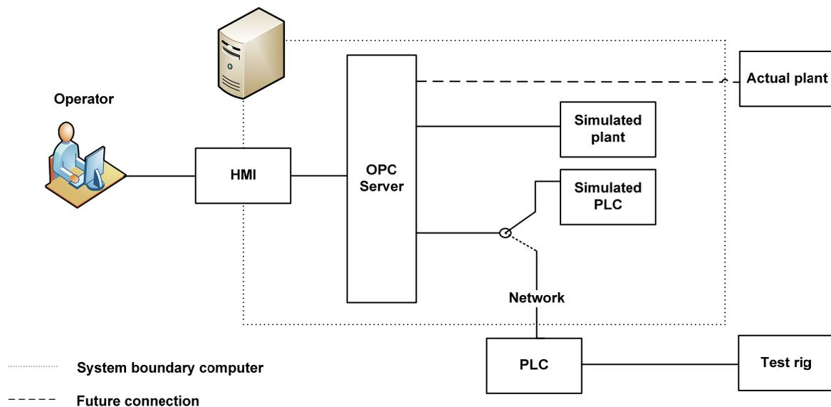
Figure 34. System architecture for enabling operator training.
