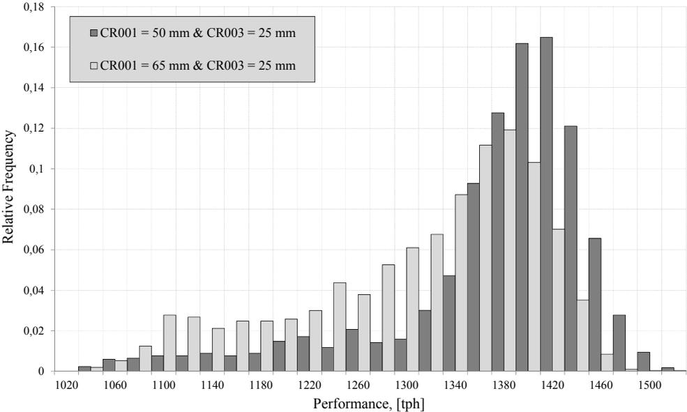
Figure 36. Plant performance for two different settings of crusher 1 (CR001).
