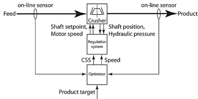
Figure 5. A closed loop process control for controlling the CSS and the eccentric speed of a cone crusher, as presented by Hulthén [10].
