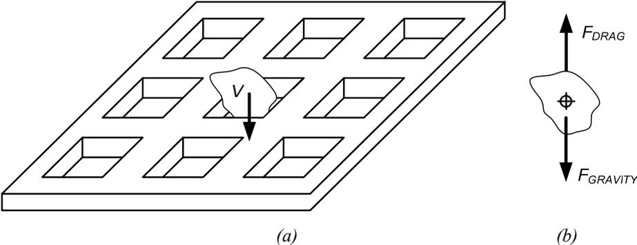
Figure 3. Two methods of separating the material with respect to certain particle size. With a fixed aperture (a) and with relative drag force (b).
