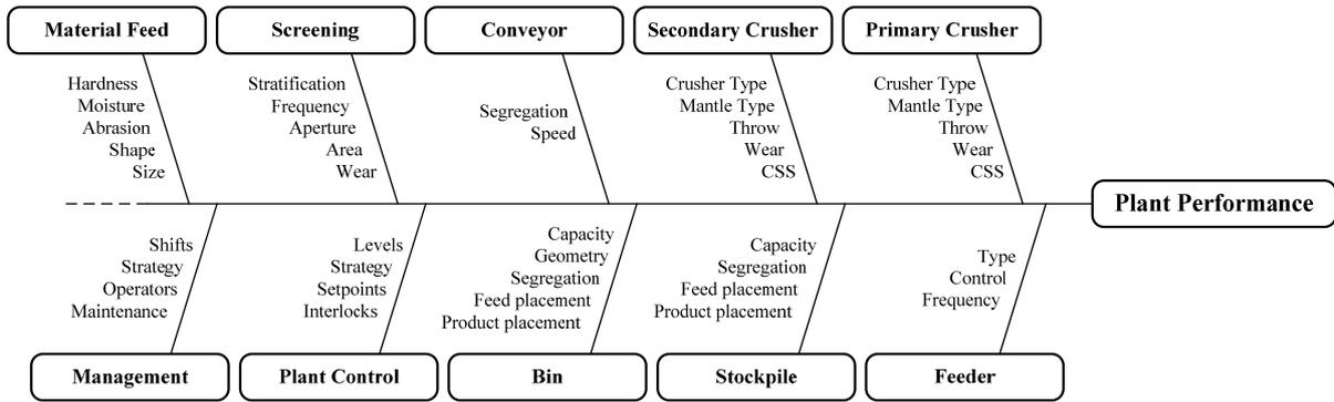
Figure 9. Cause-and-effect diagram over factors that can influence plant performance.
