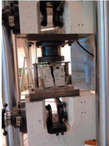
Figure 3.9. Apparatus used to determine the tensile and compressive strength of the concrete, and the failure mode of a tested cube during a tensile test.
