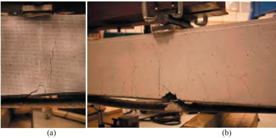
Figure E.2.11 Failure modes of beam : (a) Left side (b) Right side (Beam B9-EE1-F-C).
