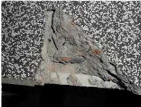
Figure E.2.4 Steel bar rupture (Beam B3-NE1-F).
