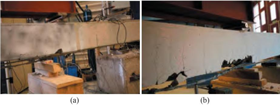
Figure E.1.9 Modes of failure of the tested beam (Beam B7-NE2-S): (a) Left side (b) Right side.
