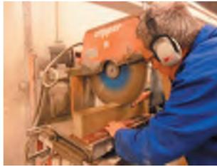
Figure 3.10. Manual sawing of the prism.
