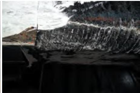
Figure E.2.7 Debonding failure (Beam B6-EE2-F).
