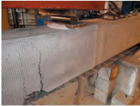
Figure E.2.3 Debonding failure (Beam B1-EE1-F).
