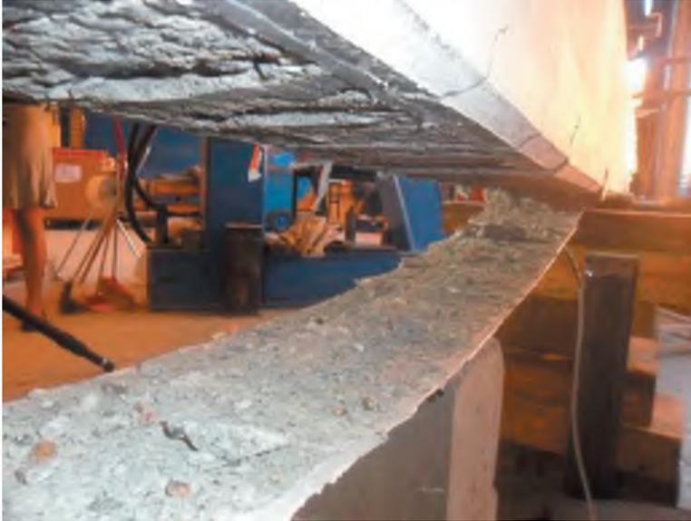
Figure E.1.3 Debonding failure (Beam B2-EE1-S).
