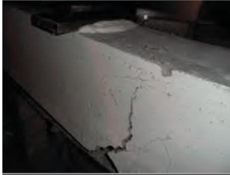
Figure E.2.2 Crush of concrete beam (Beam B1-EE1-F).
