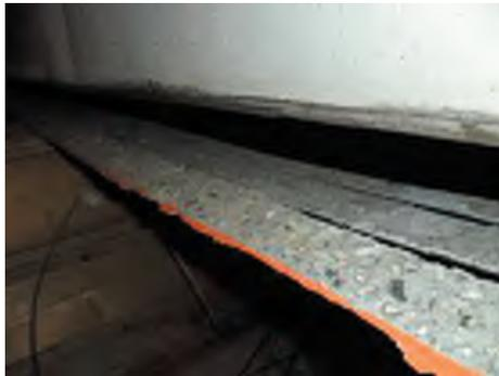
Figure E.1.7 Debonding failure (Beam B5-EE2-S).
