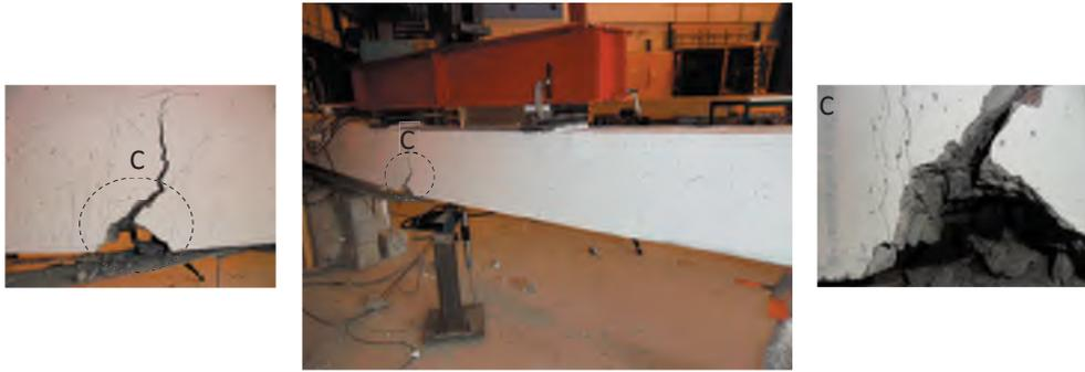
Figure 3.32. Fatigue fracture of steel reinforcing bars of Plate strengthened beam (B1-EE1-F).
