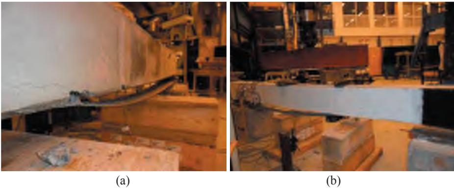
Figure E.1.6 Modes of failure of the tested beam: (a) Left side (b) Right side (Beam B5-EE2-S)
