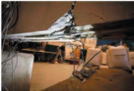
Figure E.2.14 Steel bar rupture (Beam B10-NE1-F-C).
