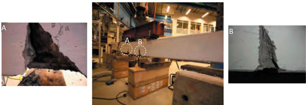
Figure 3.31 Fatigue fracture of steel reinforcing bars of NSM strengthened beam (B8-NE2-F).
