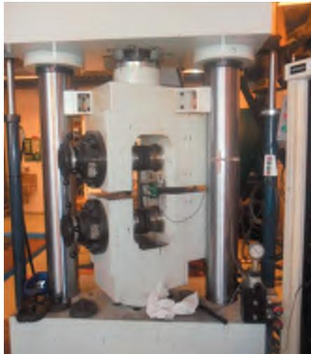
Figure 3.6. Apparatus used to determine the steel bars' mechanical properties.
