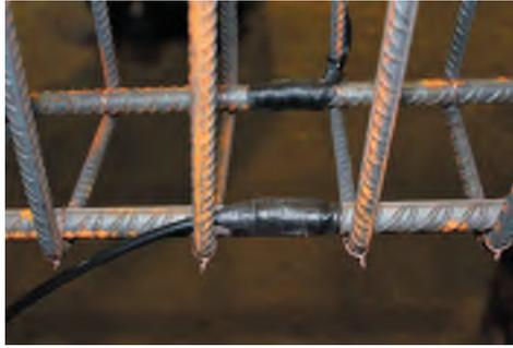
Figure 3.14. Installation of steel strain gauges.
