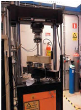
Figure 3.11. Photograph of set up used to determine the fracture energy of the concrete.
