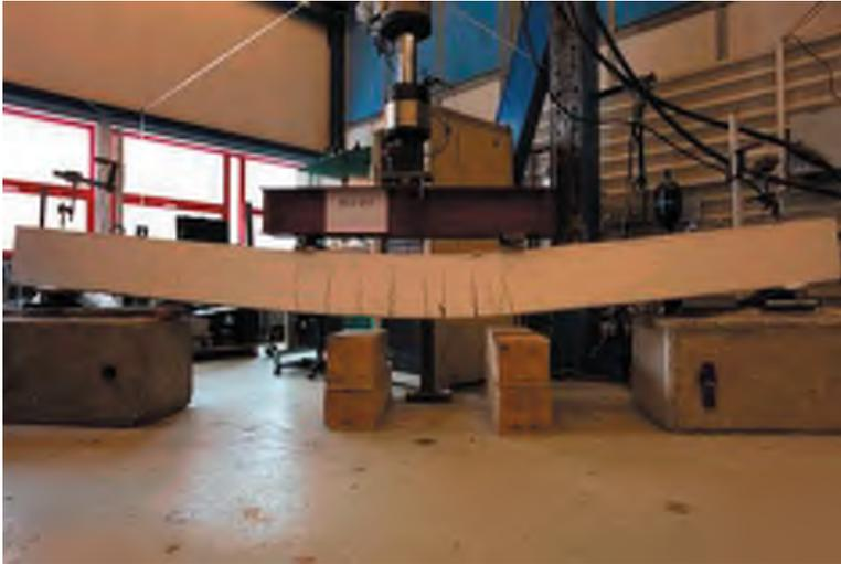
Figure E.1.1 Crushing of concrete (Beam B11-0-S).
