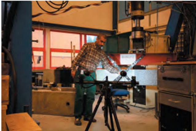
Figure 3.19. Calibration of the ARAMIS optical strain measuring system.
