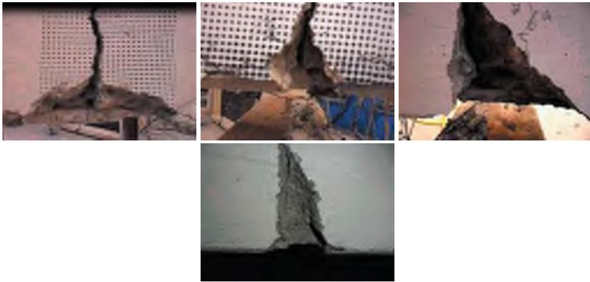
Figure E.2.9 Steel bar ruptures (Beam B8-NE2-F).
