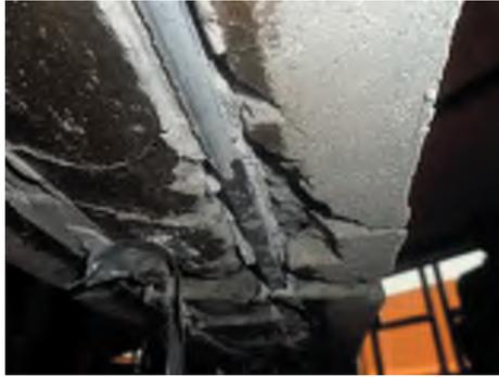
Figure E.1.5 Shear cracks along the NSM groove (Beam B4-NE1-S).
