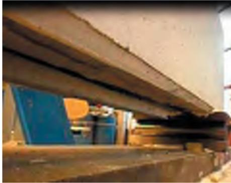
Figure E.2.10 Debonding of NSM bar (Beam B8-NE2-F).
