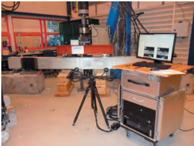
Figure 3.17. Configuration of the ARAMIS optical strain measuring system.
