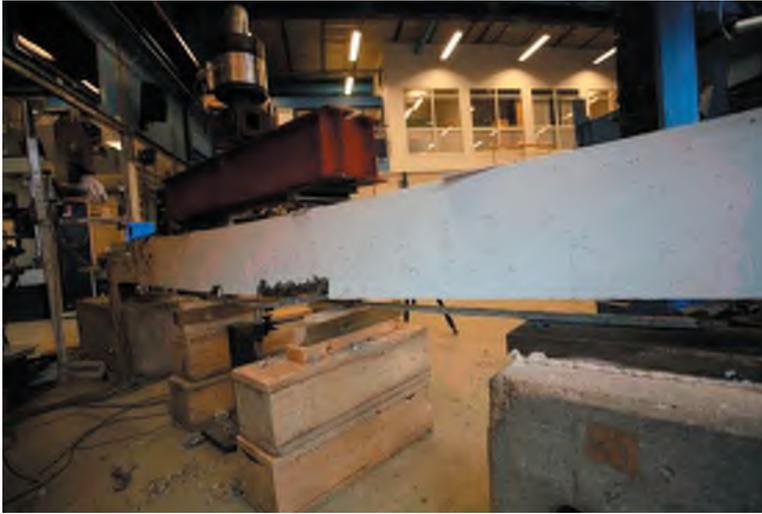
Figure E.1.8 Failure cracks pattern (Beam B7-NE2-S).
