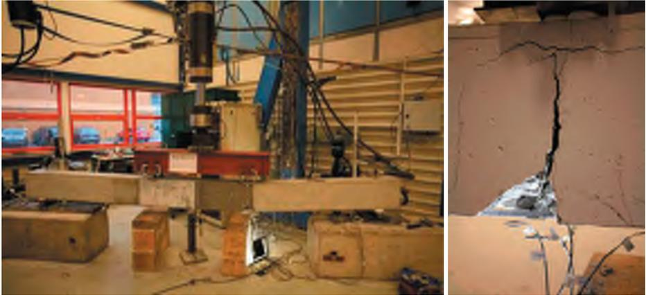
Figure E.2.13 Failure mode of beam (Beam B10-NE1-F-C).
