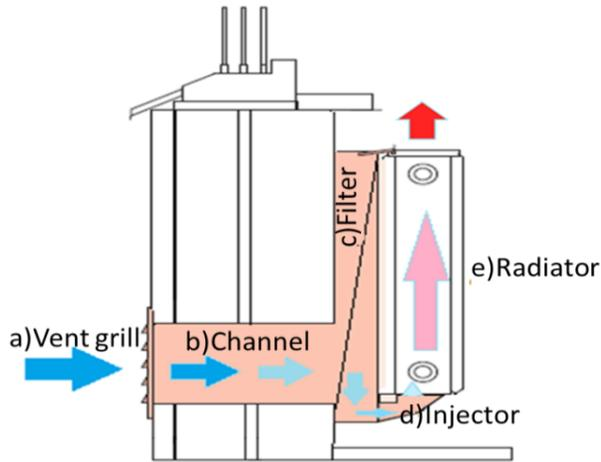
Fig. 2. Main parts of a ventilation radiator: a) Vent grill on the external wall, b) Channel through wall, c) Filter, d) Injector or inlet (with or without mixing of cold supply air with room air) e) Traditional radiator
