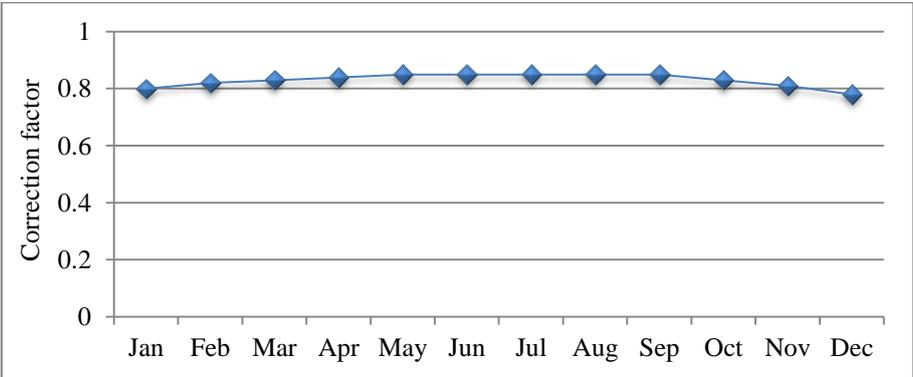
Fig. 4. Correction factor of PV output for different months (Häberlin 2012)
