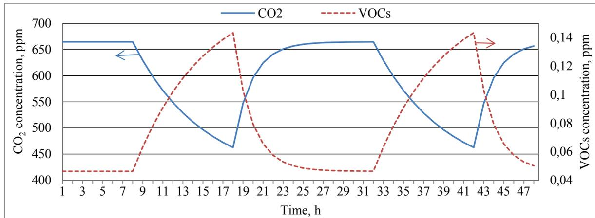
Fig. 10. Pollutant gas concentration ( $\text{CO}_2$  and VOCs) variation over 48 hours showing the effect of decreasing the ventilation rate from 8:00 till 18:00
