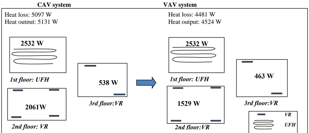
Fig. 3. Heat loss and heat output from ventilation radiators (VR) and under-floor heating (UFH) in constant air volume (CAV) and variable air volume (VAV) systems
