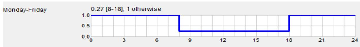
Fig. 6. Profile for the ventilation fan speed for weekdays, 1.0 for working at full power during occupancy from 18:00 till 08:00, and 0.27 for working during unoccupancy from 8:00 till 18:00 with 27 % of full speed.
