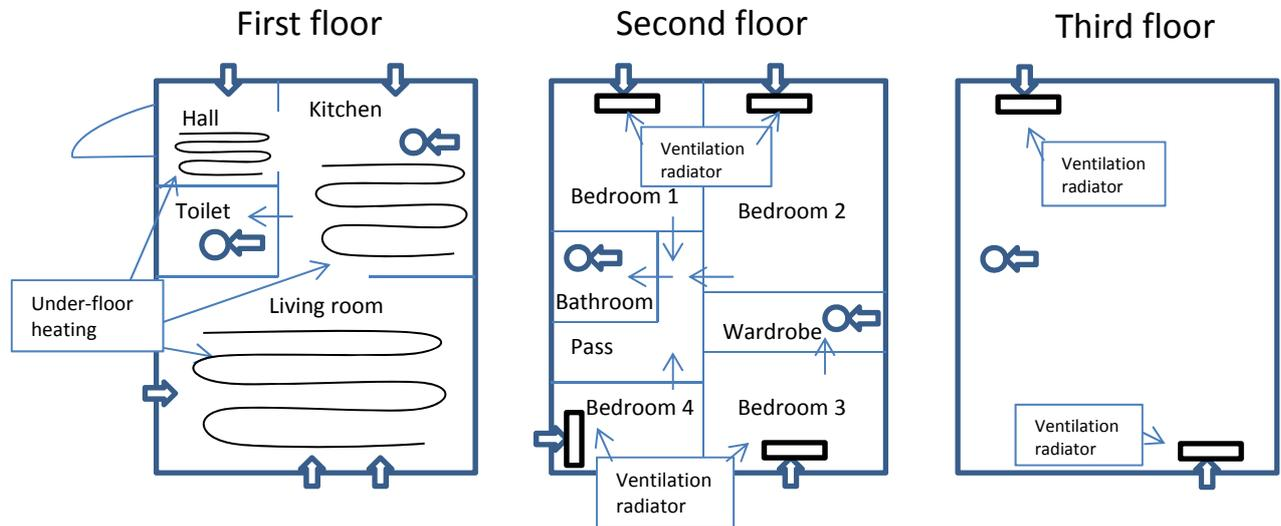
Fig. 3. Building plan and schematic of airflow and heating systems
