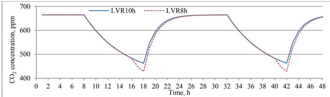
Fig. 6. Variation of CO<sub>2</sub> concentration in a room for two subsequent days based on the presence of occupants and ventilation rate for LVR10h and LVR8h
