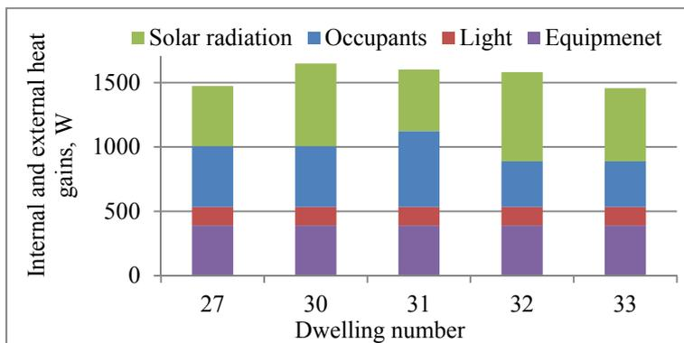
Fig. 9. Simulated internal (occupants, light and equipment) and external (solar radiation) heat gains for each dwelling
