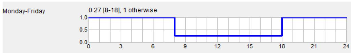
Fig. 2. Profile for the ventilation fan speed for weekdays; 1 for working in full power during occupancy (18:00-8:00) and 0.27 for working with 27 % of full speed during unoccupancy (8:00-18:00)
