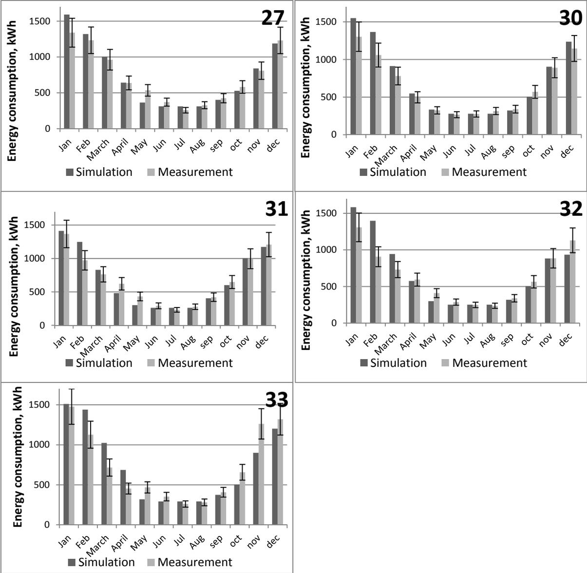
Fig. 7. Comparison between measured and calculated energy consumption for the five houses studied
