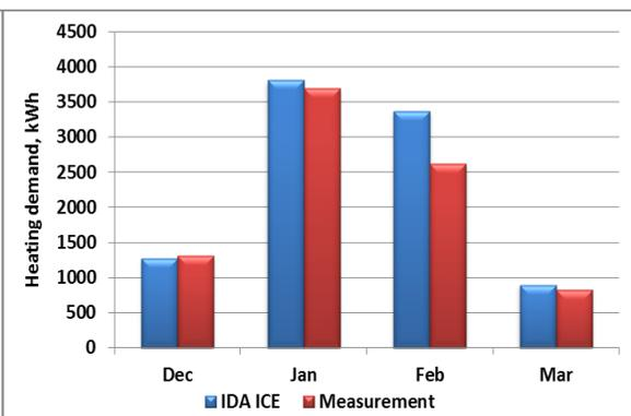
Figure 6. Comparison between site measurements and simulation results by IDA ICE
