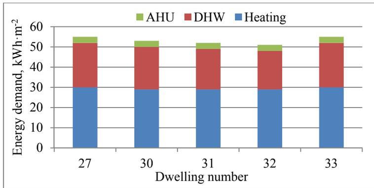
Fig. 8. Measured energy consumption for each dwelling for air handling unit (AHU), domestic hot water (DHW) consumption and heating system
