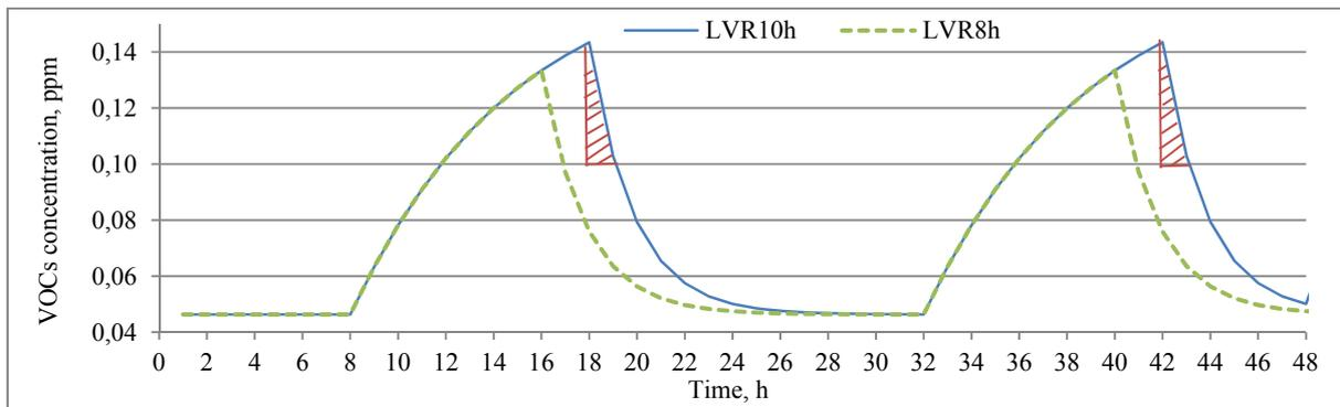
Fig. 5. VOC concentration in a room during two subsequent days for LVR8h and LVR10h showing the influence of flow rate reduction during unoccupancy on VOC concentration; the periods for LVR10h with greater concentration than allowable when occupants are home are marked in red.
