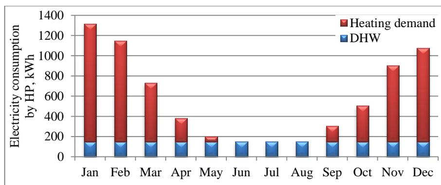
Fig. 2. Monthly electricity consumption of a heat pump with COP 02.7
