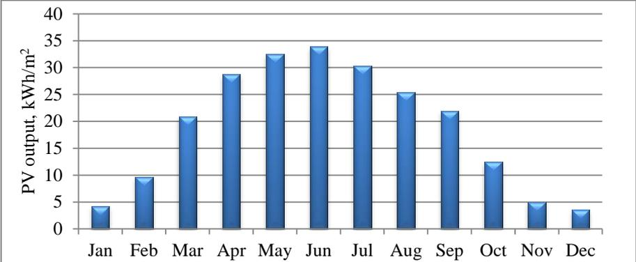
Fig. 3. Photovoltaic output at 15 % efficiency in Stockholm
