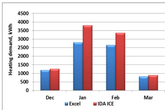
Figure 5. Comparison of results from energy balance calculation in Excel and IDA ICE simulations
