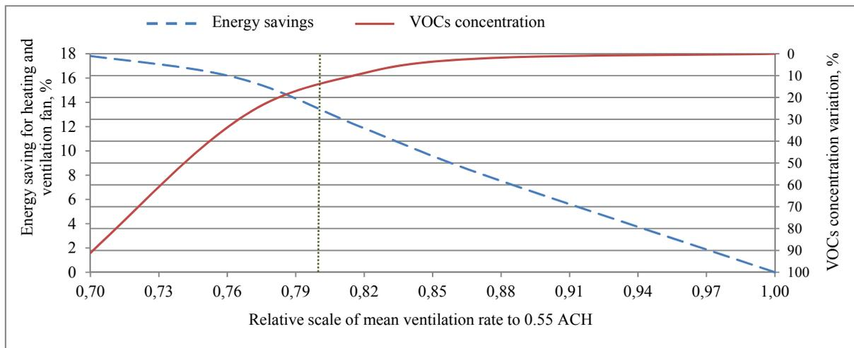
Fig. 8. Energy savings and VOC variation in percent of total concentration for different mean ventilation flow rates
