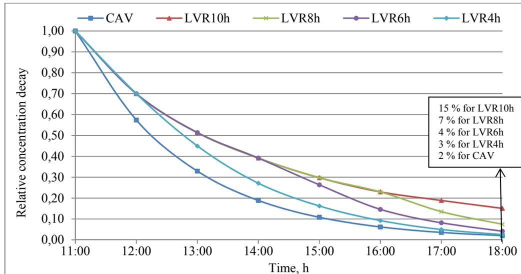
Fig. 4. Relative concentration decay for different VAV durations showing the concentration levels during seven hours before 18:00, i.e. when occupants arrive home
