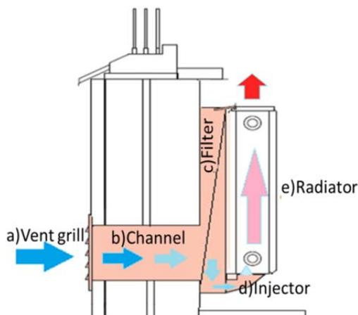
Fig. 2. Main parts of a ventilation radiator: a) Vent grill on the external wall, b) Channel through wall, c) Filter, d) Injector or inlet (with or without mixing of cold supply air with room air) e) Traditional radiator
