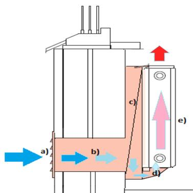
Figure 2. Main parts of ventilation radiator: a) Vent grill on the building wall b) Channel through wall c) Filter d) Injector or inlet (with or without mixing of cold supply air with room air) e) Traditional radiator (Myhren 2011)
