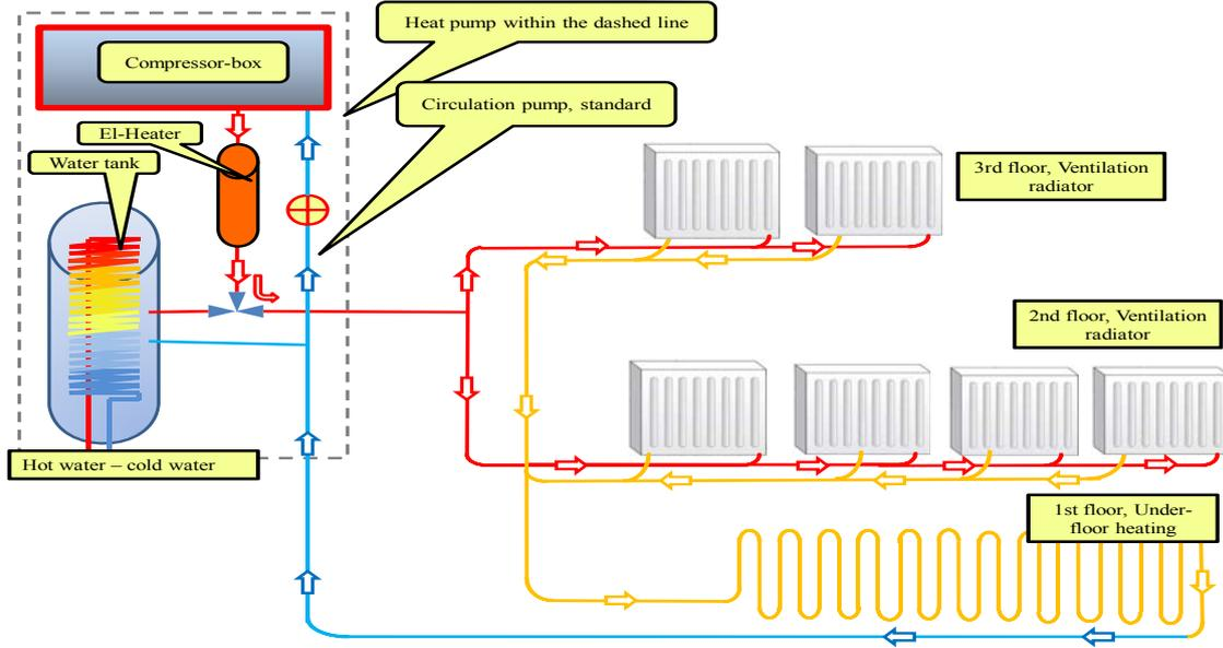
Fig. 4. Low-temperature hydronic heating system connected to the heat pump and water tank for producing domestic usage
