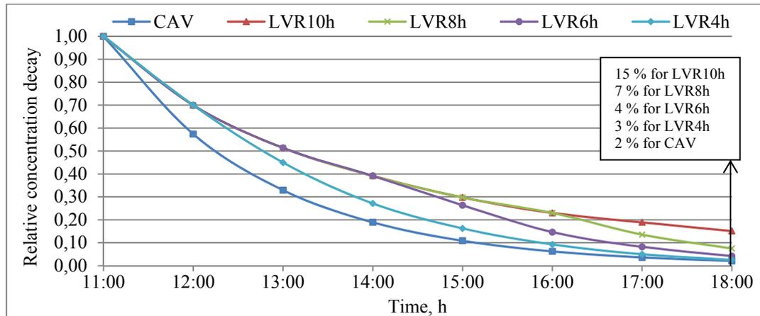
Fig. 11. Relative concentration decay for different VAV durations showing the concentration level seven hours before 18:00, i.e. when occupants arrive home
