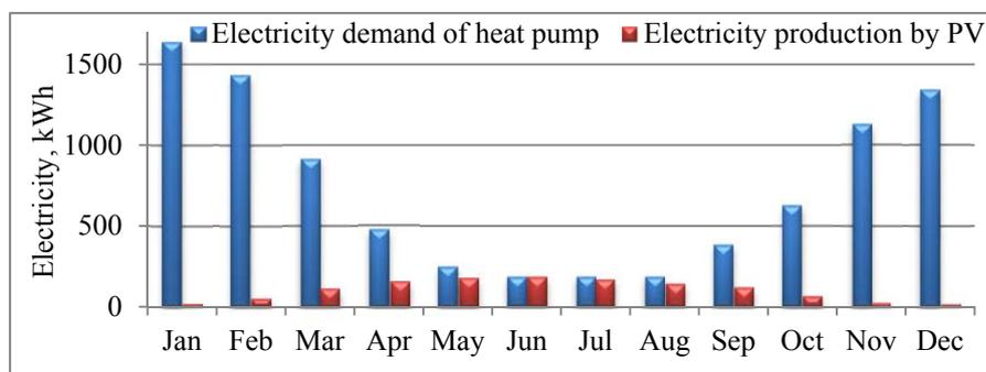
Fig. 12. Simulated monthly electricity demand of heat pump and electricity production by 7 m<sup>2</sup> PV
