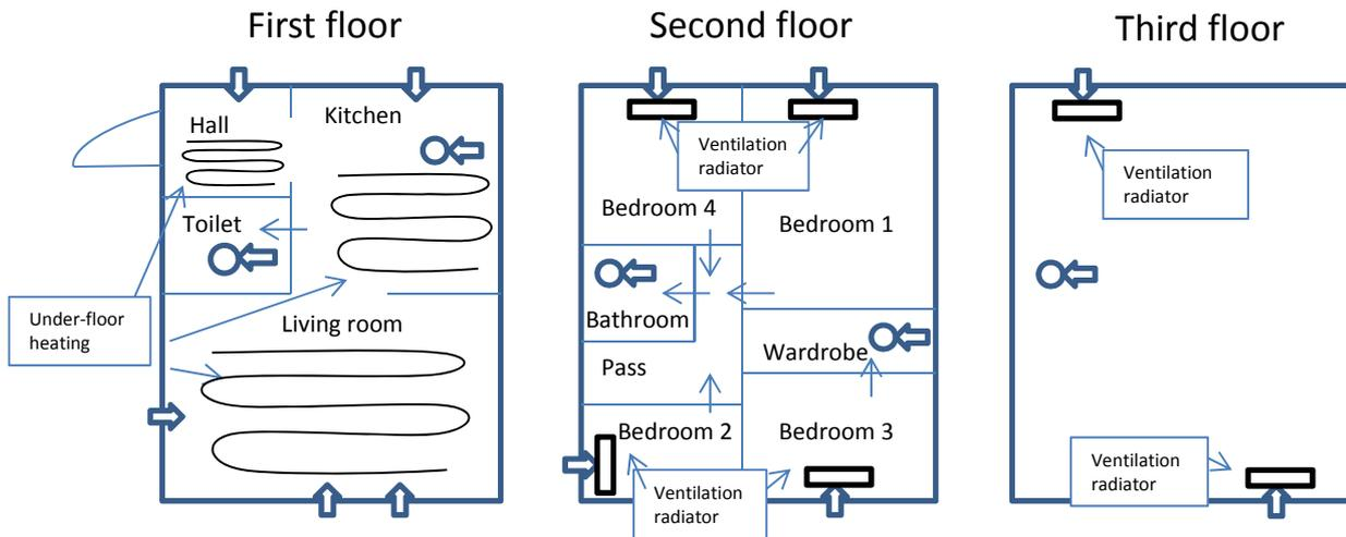
Fig. 1. Building plan showing the schematic of airflow and heating systems
