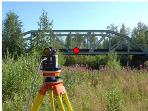
Figure 6.6 Position of the laser targeting the prism placed on the truss in the middle of the bridge
