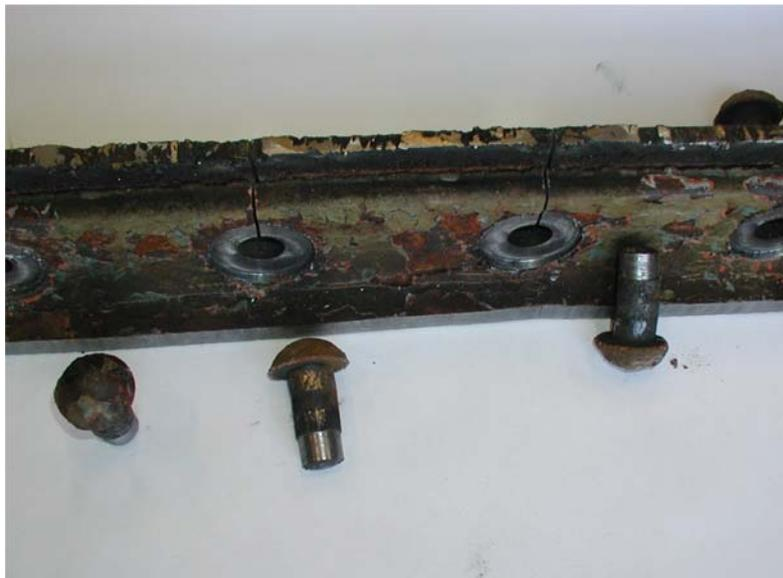
Figure 4.5 The part of the web connected to the “flanges” cut out to be able to extract the rivets for tensile testing
