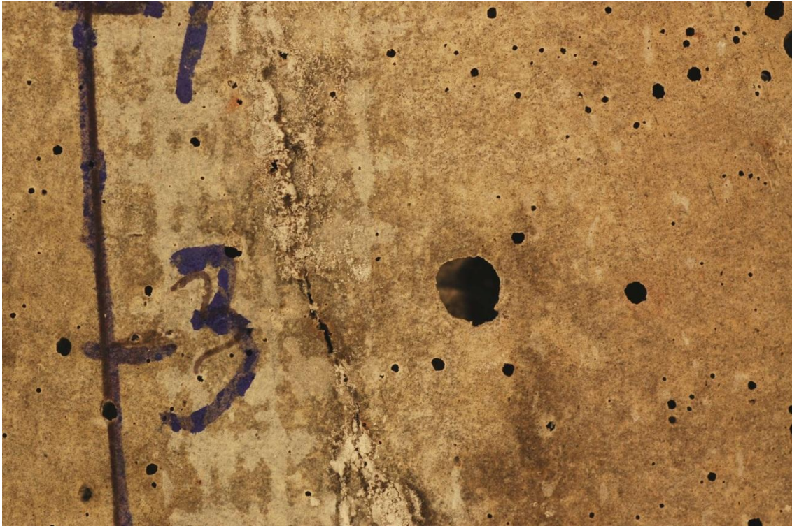
Figure A2.1: 0.2 mm crack after 1 year permanent immersion in sea water. Test series 1, specimen H75-2-1-1.
