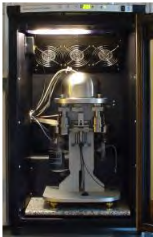
Figure 1. On the left side the sorption balance in a climate cabinet from Surface measurements System, SMS, is shown on the right side a sorption balance principle is shown
