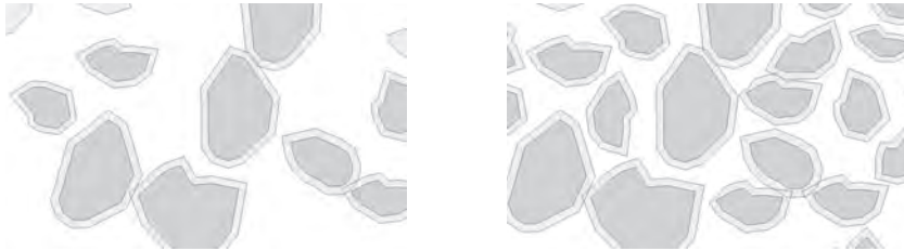
Figure 2.2: Illustration of a high water cement ratio to the left and a low water cement ratio to the right. Water, reaction products (C-S-H gel and others), and cement grains are represented by the white area, lighter and darker shaded polygons respectively.
