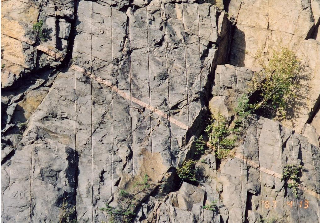
*Figure 5.9 Typical intrusion of magma in gneiss of igneous origin that was once located deep down in the crust of the earth. Grout-stone intrusions observed in excavations in grouted rock usually have an identical appearance.*
