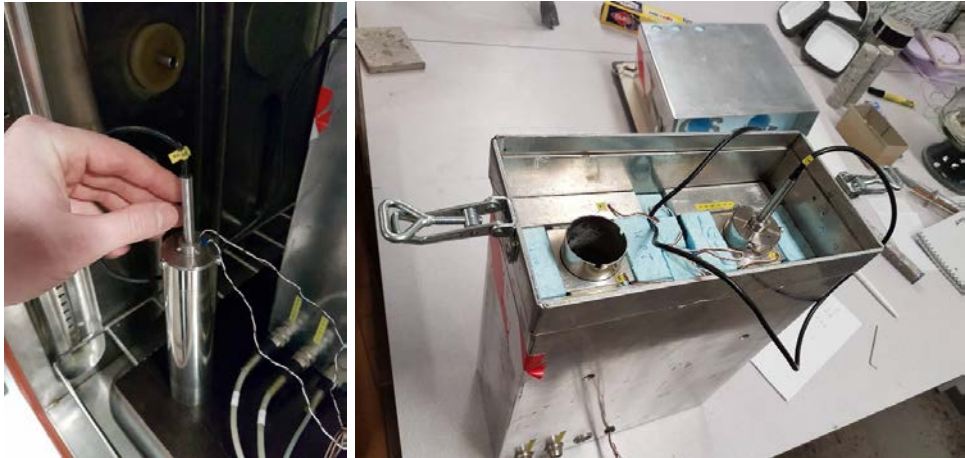
Figure 9. Calorimetry and dilation experimental set-up. An LVDT gauge is placed on top of the sample through the lid of the invar vessel (left). Invar vessel placed in one of the vessel holders of the instrument.
