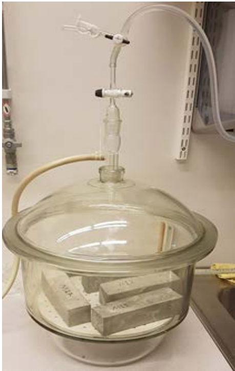
Figure 7. Porosity measurement, showing dried samples under vacuum; samples are later covered in deionized water.
