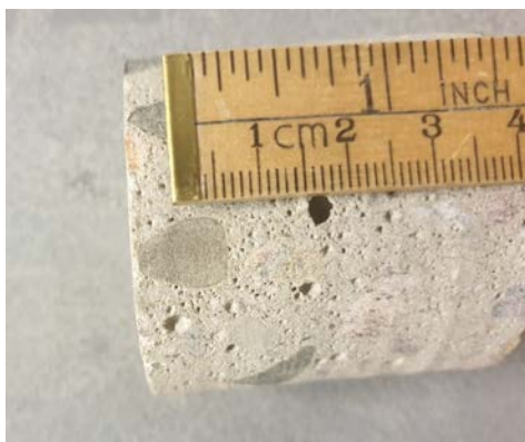
FIGURE 9 EXAMPLE OF LARGER AIR VOIDS ON SURFACE OF CONCRETE SAMPLE, MEASUREMENTS WERE MADE ON 5 SAMPLES FROM EACH MATERIAL.
