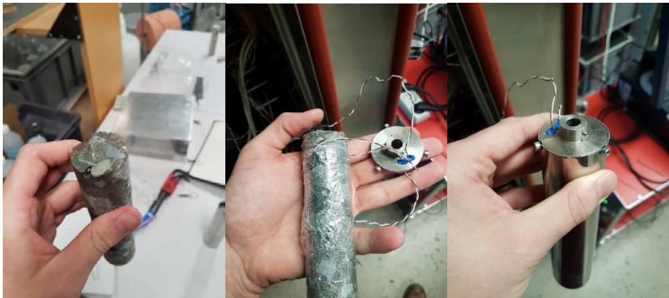
Figure 8. Calorimetry and dilation experimental set-up. Sample with a piece of glass glued on top, to ensure free movement of the LVDT (left). Sample with a thermocouple on the surface of the sample and sealed with plastic (Middle). The sealed sample placed in an invar vessel (right).
