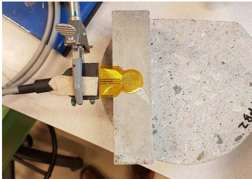
Figure 6. Hot disk measurement, showing the sensor placed on the mortar prism. During the measurement, the sensor is placed between the prism and an EPS-insulation.
