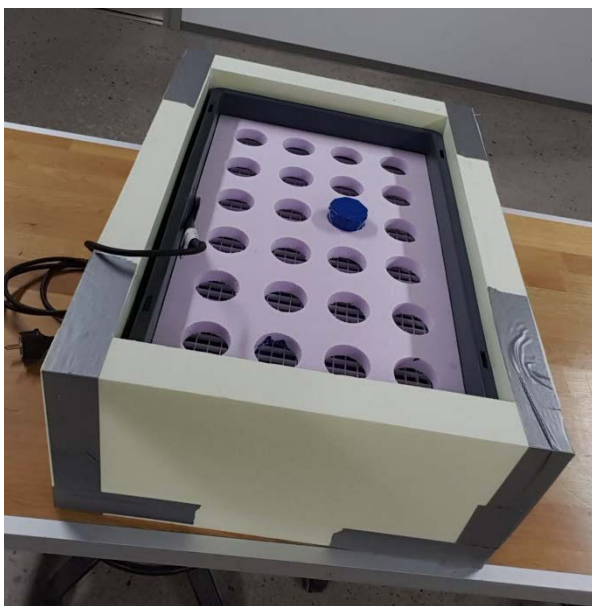
FIGURE 1 SET-UP FOR -20\text{ }^{\circ}\text{C} AND FOR CYCLING BETWEEN +20 AND -20\text{ }^{\circ}\text{C} WITH ONLY ONE SAMPLE INSERTED.
