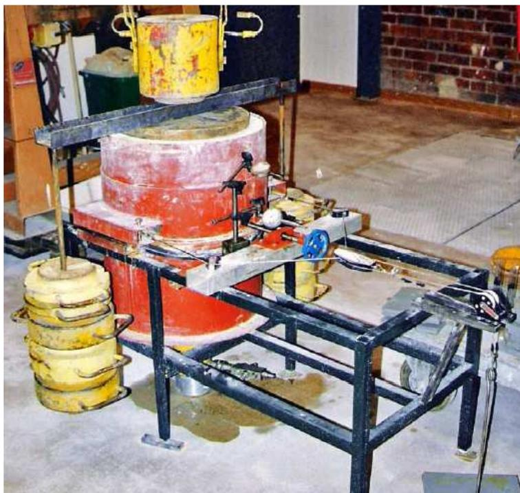
Figure 2.5: Shear box apparatus. From Larsson (2008).
