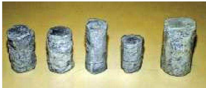
Figure 4.5: Samples before the unconfined compression tests. From Larsson (2008).
