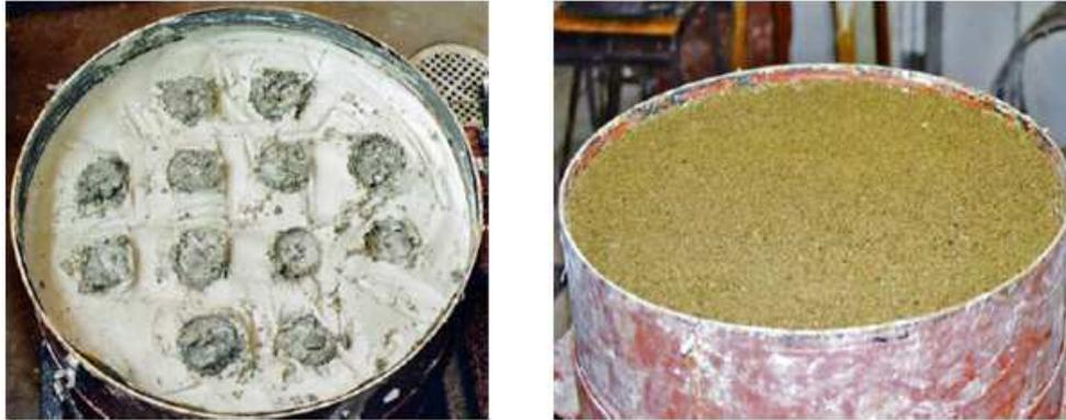
Figure 2.2: Top surface without and with a 50 mm thick sand layer. From Larsson (2008).
