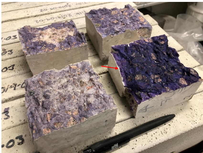
Figure 4.30. Cubes of CH-S65 after being split and checked for carbonation imprints before initiation of accelerated carbonation test. Only very vague carbonation is noticeable on the surface/side of one of the cubes (red arrow).
