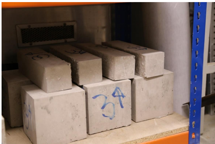
Figure 4.14. Concrete cubes and prisms (300 mm in length) resting on top of cubes prior to being cut in two halves for radon gas measurements.
