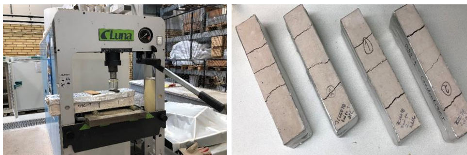
Fig 4.28. (a) Luna pressure press used to induce cracks in concrete prisms. (b) The concrete prism with cracks induced. The first two prisms to the left are from recipe one (C) and the other ones are from recipe two (C-H1).
