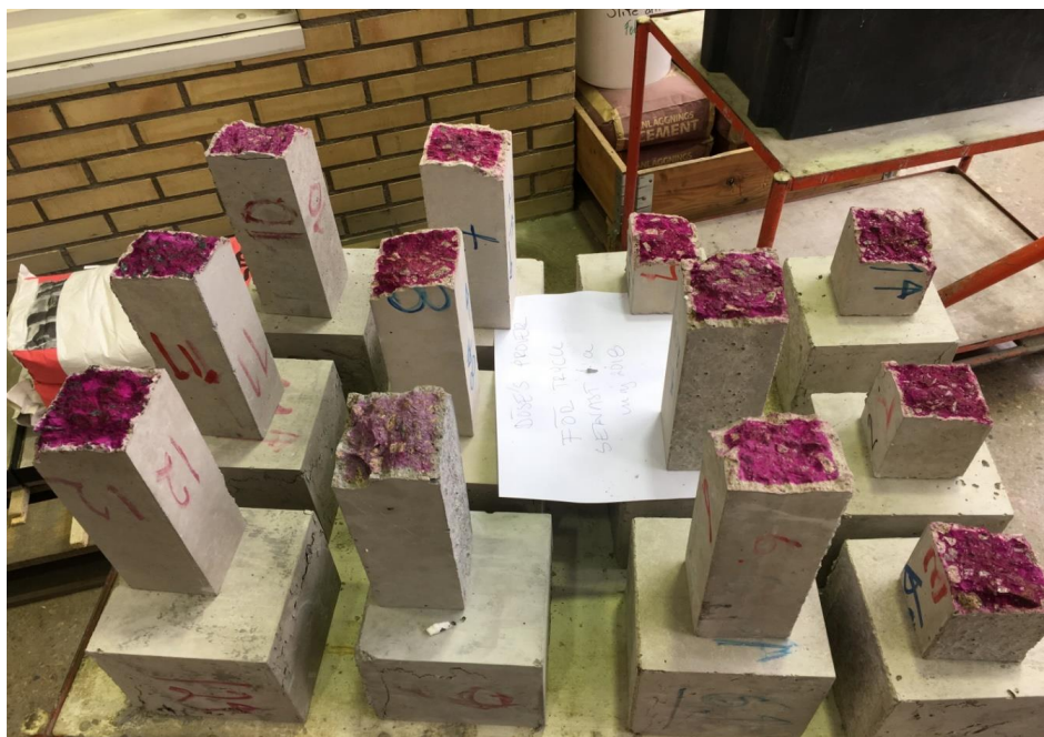
Figure 5.18. Different concrete castings of the 12 recipes with different carbonation depths. The samples are shown numbered 1-12, in columns, from the upper right corner to the lower left corner.
