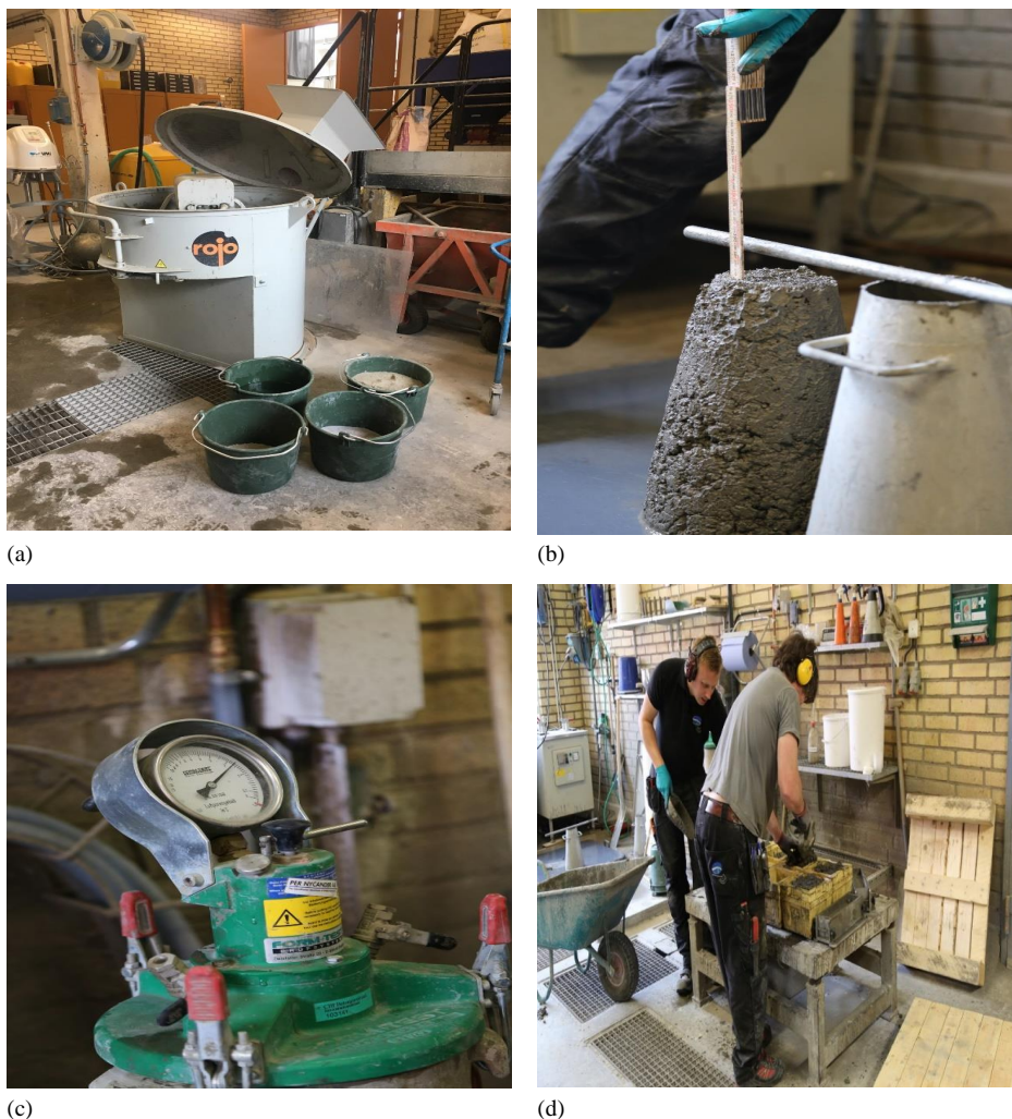
Figure 4.11. (a) Green buckets containing different binders before mixing with the Rojo concrete mixer/blender. (b) Measurement of slump after casting. (c) Measurement of the air content in the concrete using the pressure gauge method. (d) One concrete recipe being placed in molds prior to vibration.
