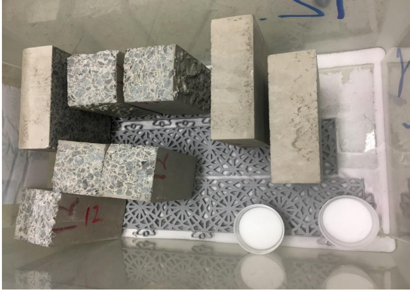
Figure 4.15. Concrete prisms and cut concrete plates (recipe CGB) in their first drying phase to reach approximate equilibrium of RH 75 %. Extra salt is also noted in two small plastic containers.
