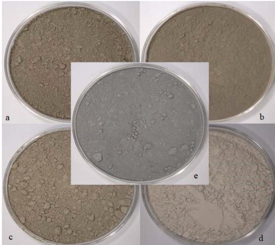
Figure 4.8. Five different SCMs/binders used in the recipe's. (a) Fly ash, (b) Micro fly ash, (c) Cement (Skövde CEM I-SH 52.5 R). (d) Slag from Bremen and in the middle (e) Micro silica – 940.
