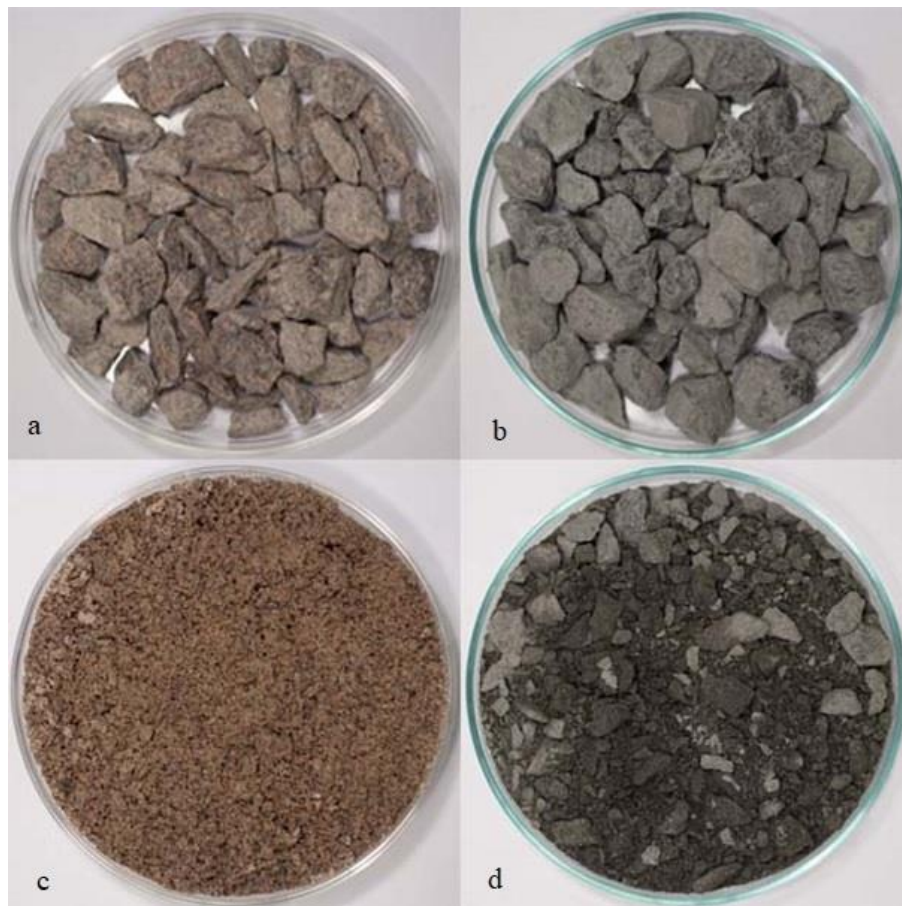
Figure 4.9. Aggregates used in the recipes. (a) Red granite, particle size fraction 8-16 mm. (b) Grey-black diabase/gabbro, particle size fraction 8-16 mm. (c) Red granite, particle size fraction 0-5 mm. (d) Grey-black diabase/gabbro, particle size fraction 0-8 mm.
