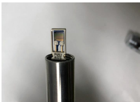
Figure 4.18d. Close up of the humidity sensor as shown in Figure 4.18a with the protective cover taken off.
