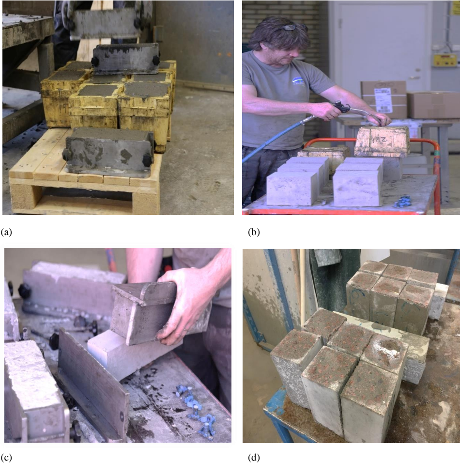
Figure 4.12 (a) Concrete cubes and prisms on a pallet after vibrating. (b) Demolding of the concrete cubes after 24h of hydration using air pressure to release the molds. (c) Demolding of concrete prisms resting on a carriage. (d) Prisms, after being cut in two halves resting on a carriage.
