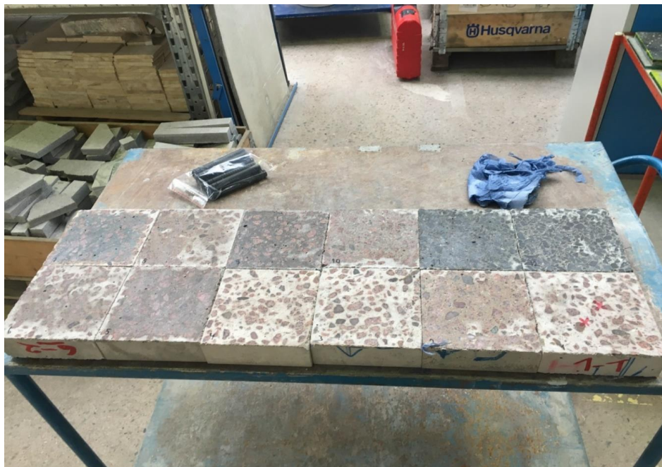
Figure 4.13. Cut samples from the cast concrete cubes resting on a carriage. The “measurement plates” constitutes one plate from each of the recipes (all in all, 12 different concrete recipes). From lower right corner to upper right corner the recipes numbered from 1-12 are shown clockwise.
