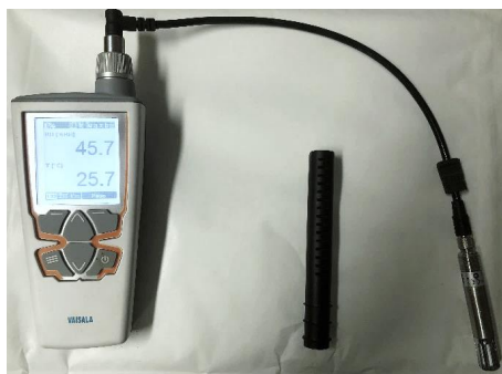
Figure 4.18c. Monitor from Vaisala Oy connected to the humidity sensor in the lower right corner. In the middle: the black hollow plastic pipe that is mounted into the concrete.
