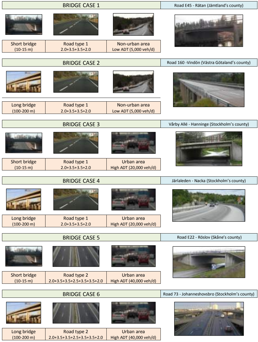
Figure 26: The six bridge cases accounted in the LCCA with a Swedish bridge example for each case
