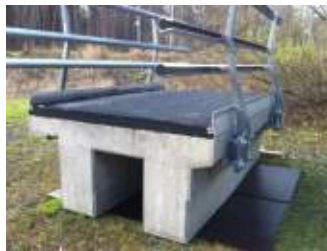
Figure 52: Prototype of a solution without an edge beam for a bridge deck with an overhang (left part) and a frame bridge (right part)
