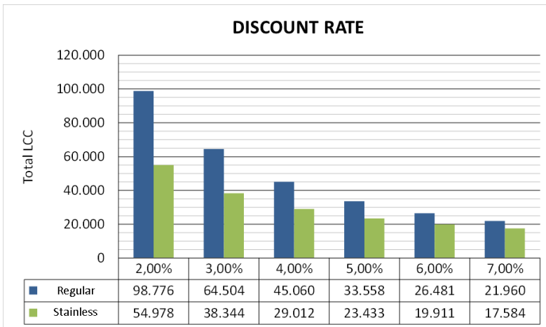
Figure 30: The influence of the interest rest on the total LCC for bridge case 6 using the design solution Type I with regular steel and with stainless steel
