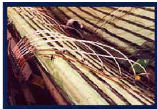
Clear tubes connect the resin distribution manifold, on the left side, to the resin feeder lines (dark-colored lines) along the hull half.
