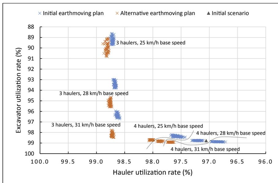
**Fig. 9.** Utilization rates of used equipment in the initial scenario and Eco-Hauling scenarios relating to number of vehicles, base speed, and anticipation of obstacles for the Initial and Alternative earthmoving plans.
