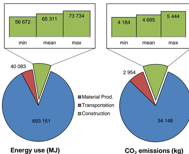
**Figure 4.** The energy use and CO<sub>2</sub> equivalent emissions of each category.
