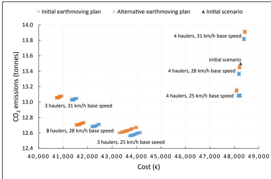
**Fig. 8.** Diesel-based fuel use and costs of the initial scenario and Eco-Hauling scenarios relating to number of vehicles, base speed, and anticipation of obstacles for the Initial and Alternative earthmoving plans.
