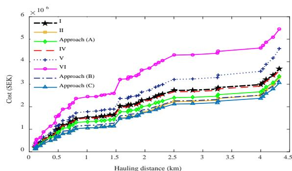
**Fig. 13. Cumulative earthmoving costs per configuration.**
