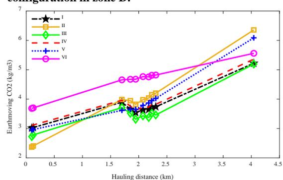
**Fig. 8. CO<sub>2</sub> emissions per unit of mass hauling by configuration in zone E.**
