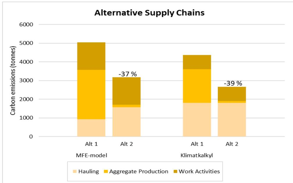
Figure 12. Predicted carbon emissions for two supply chain configurations generated using the MFE-model and Klimatkalkyl.
