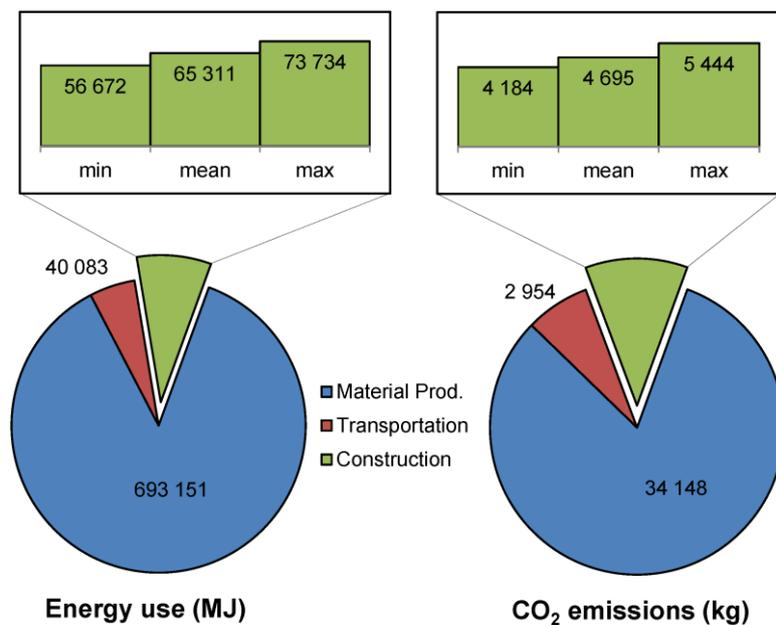
Figure 7. The energy use and carbon emissions of the upstream processes required to construct the bridge superstructure.
