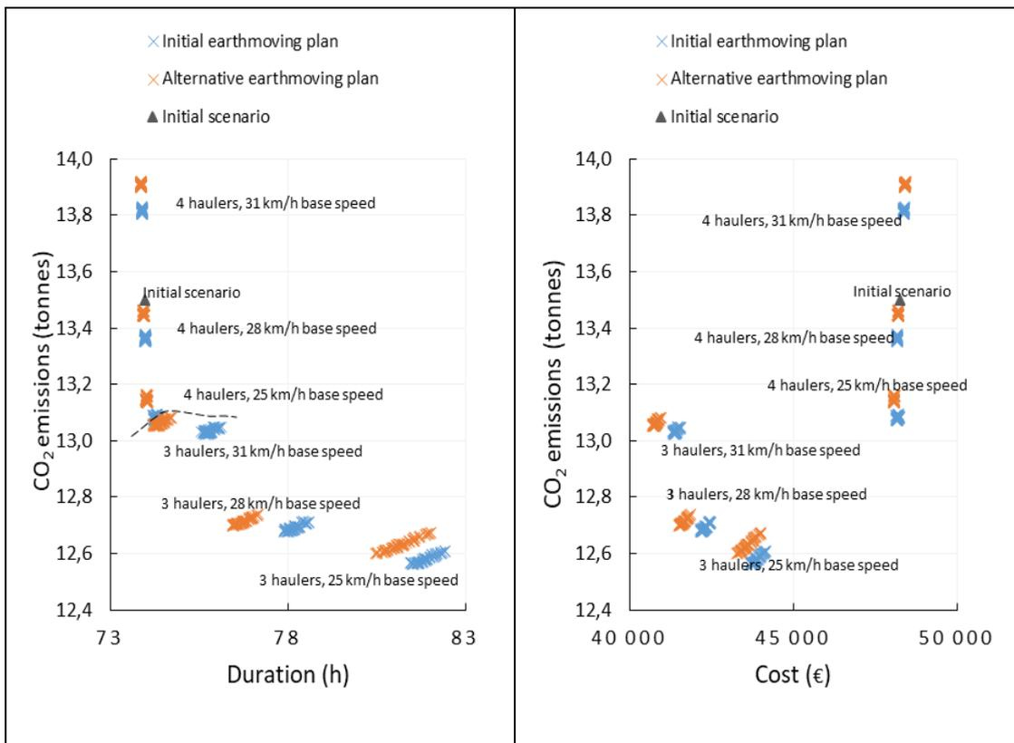
Figure 8. The results of all studied combinations of Eco-Hauling scenarios (except those using HVO) with respect to CO<sub>2</sub> emissions, duration, and costs.
