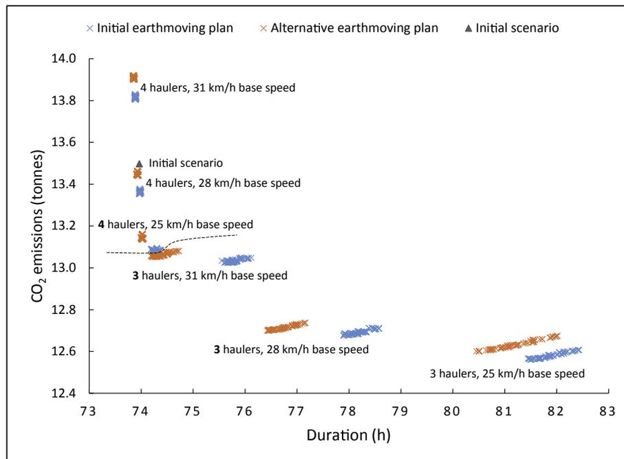
**Fig. 7.** Diesel-based CO<sub>2</sub> emissions and duration of the initial scenario and Eco-Hauling scenarios relating to number of vehicles, base speed, and anticipation of obstacles for the Initial and Alternative earthmoving plans.
