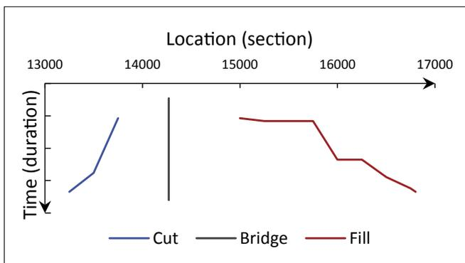
**Fig. 5.** The earthmoving plan of the initial scenario.
