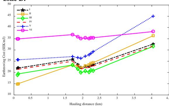
**Fig. 7. Cost per unit of mass hauling by configuration in zone E.**
