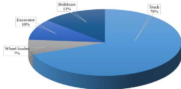
Fig. 12. Weighted ratio of CO<sub>2</sub> emissions by equipment type.
