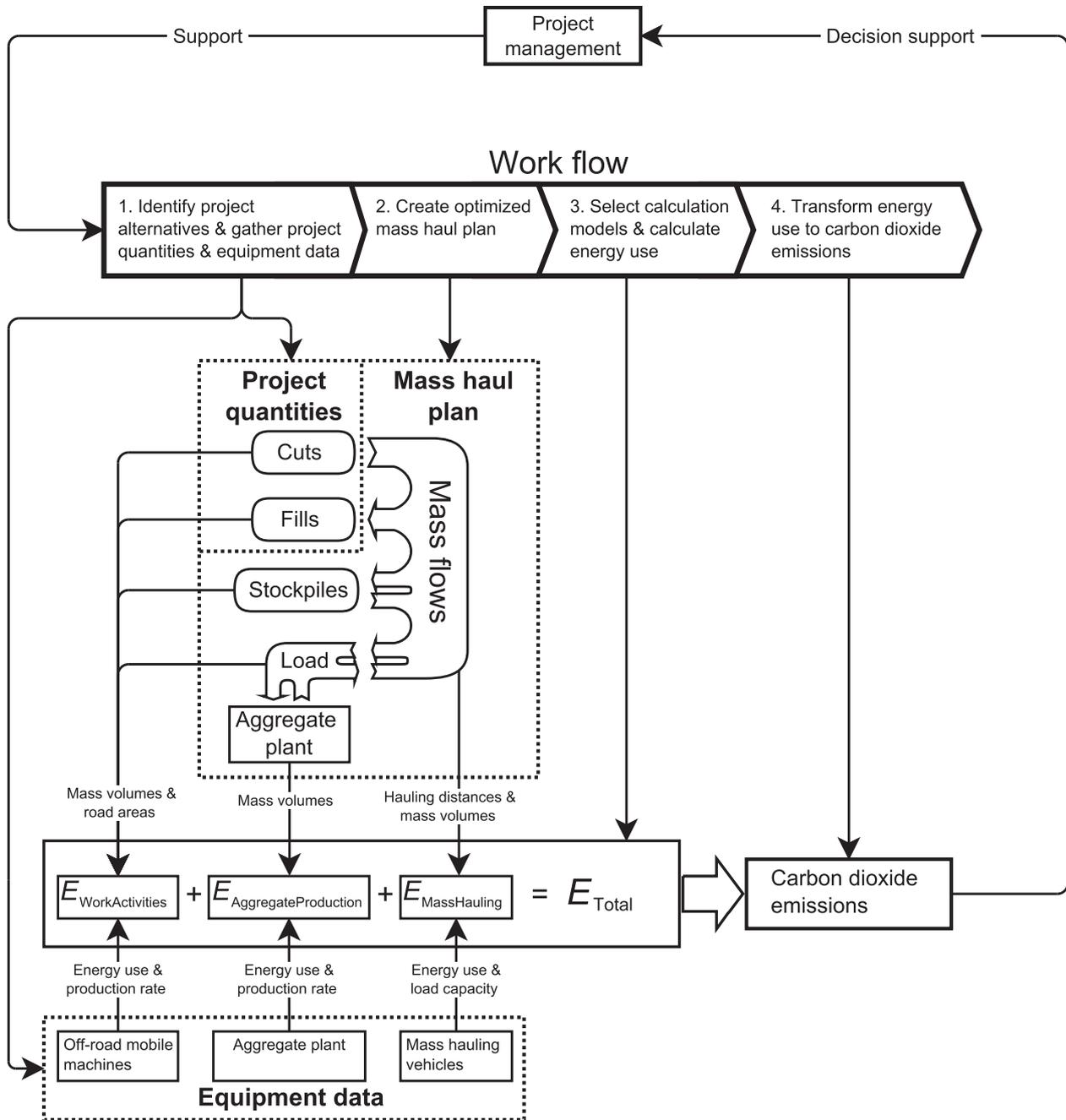
Fig. 1. The mass flow emissions (MFE) model.
