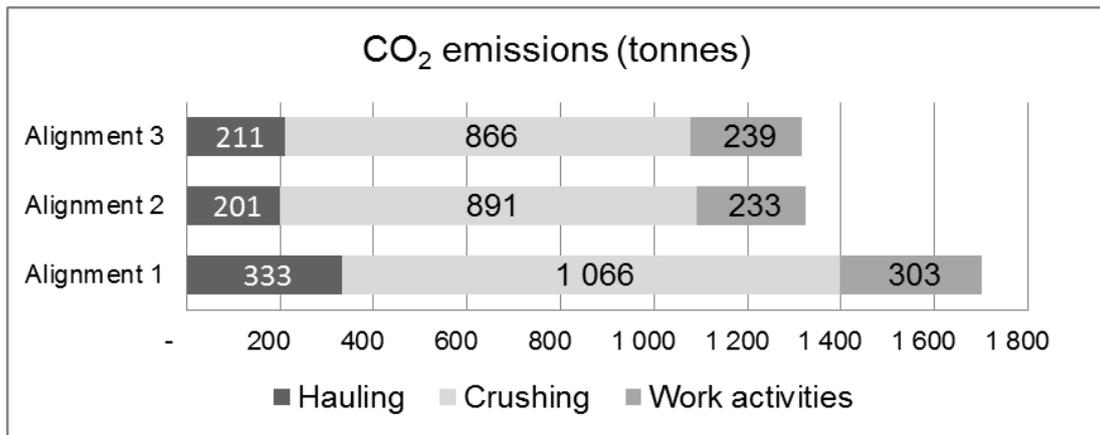
**Figure 3. Case study results with CO<sub>2</sub> emissions of each alignment.**
