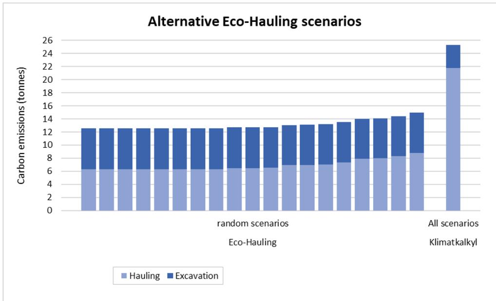
Figure 13. Predicted carbon emissions for a number of randomly chosen scenarios generated using the Eco-Hauling method and Klimatkalkyl.
