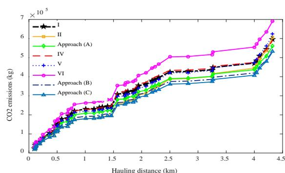
**Fig. 14. Cumulative earthmoving CO<sub>2</sub> emissions per configuration.**
