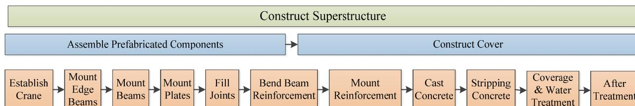
**Figure 2.** Construction process of the bridge superstructure.
