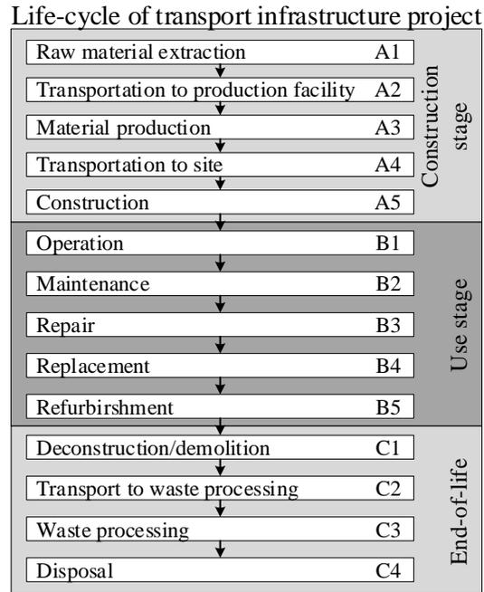
*Figure 3. Life-cycle stages of a transport infrastructure project. Adapted after Strömberg (2017) and the International EPD System (2012) and (2013).*
