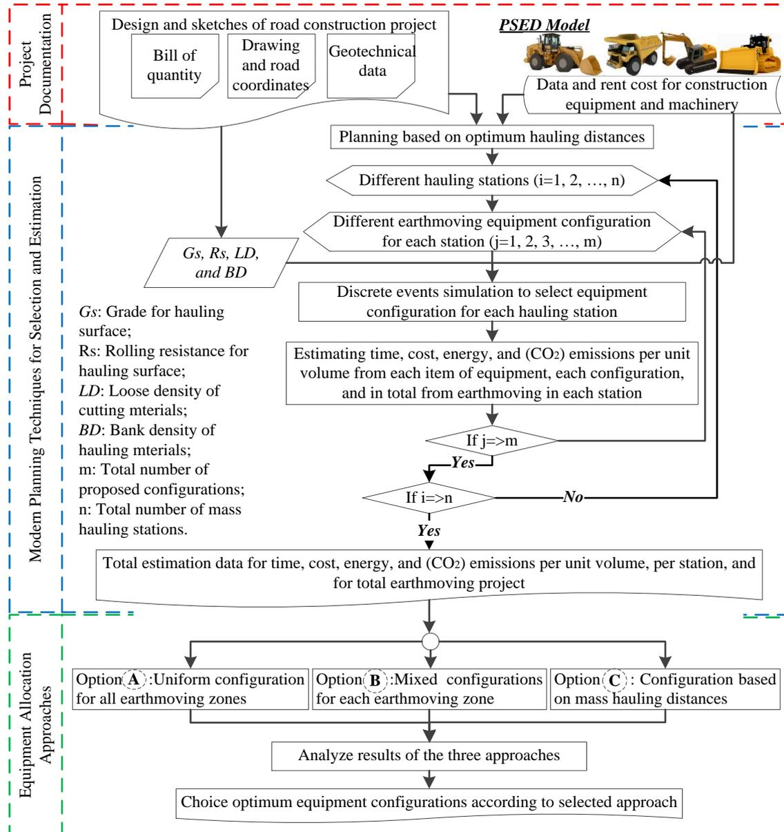
Figure 9. Outline of the Planning, Simulation, Estimation, and Decision making (PSED) model and its implementation.
