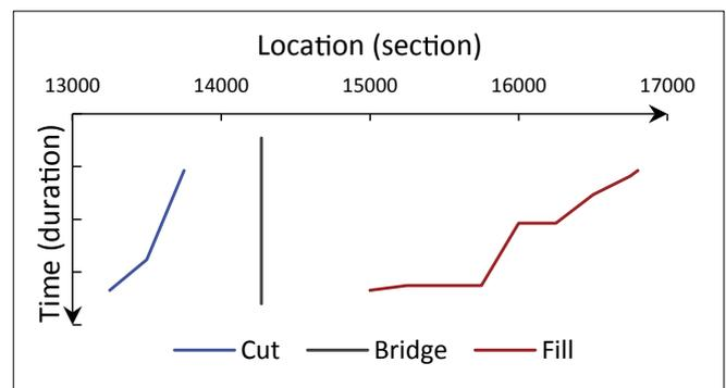
**Fig. 6.** The Alternative earthmoving plan of Eco-Hauling.
