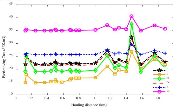
**Fig. 9. Cost per unit of mass hauling by configuration in zone I.**
