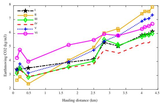
**Fig. 6. CO<sub>2</sub> emissions per unit of mass hauling by configuration in zone D.**
