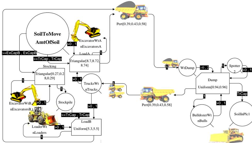
Fig. 4. Example of earthmoving simulation template used.
