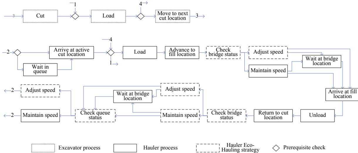
**Fig. 4.** The earthmoving process logic with Eco-Hauling.
