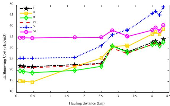
**Fig. 5. Cost per unit of mass hauling by configuration in zone D.**
