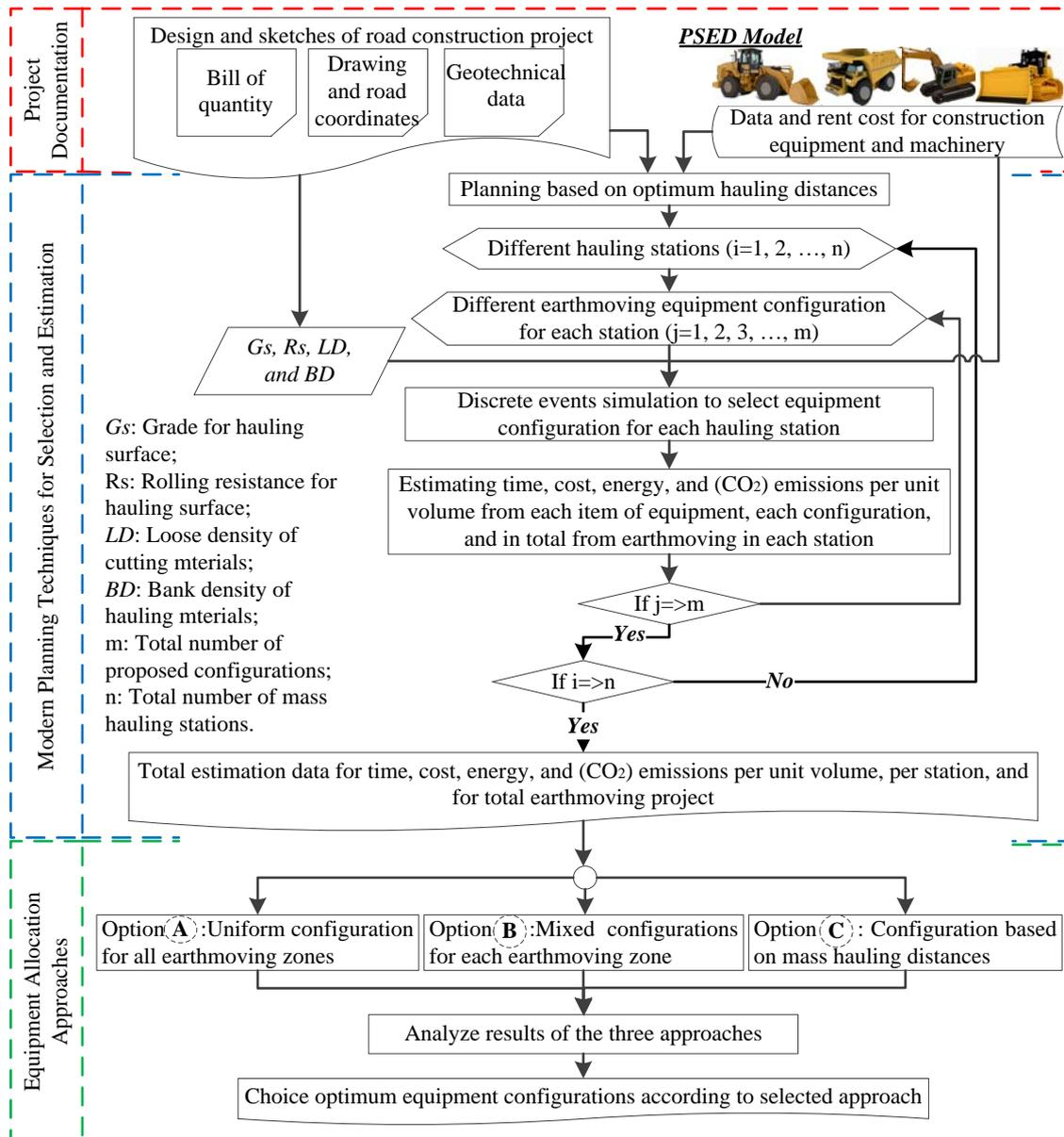
Fig. 1. Outline of the Planning, Simulation, Estimation, and Decision making (PSED) model.
