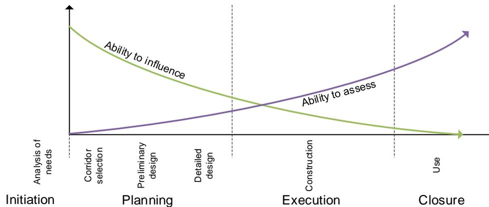
Figure 2. Schematic illustration of the ability to influence project parameters during different stages in transport infrastructure projects. Adapted after Trafikverket (2017a) and Paulson (1976).
