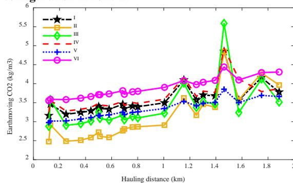
**Fig. 10. CO<sub>2</sub> emissions per unit of mass hauling by configuration in zone I.**
