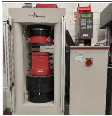
Figure 11: Compressive strength testing machine.
