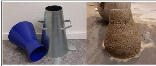
Figure 9: The slump test setup used to determine the workability of concrete.
