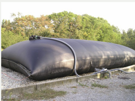
Figur 1. Geotub under tryck.
