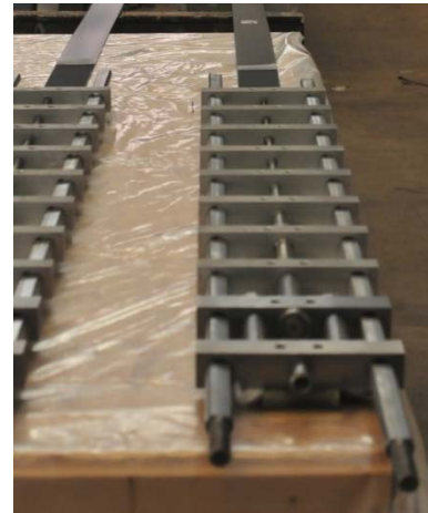
Fig. 4.2 Mounted pre-stressing device to the CFRP ready to be used on site.
